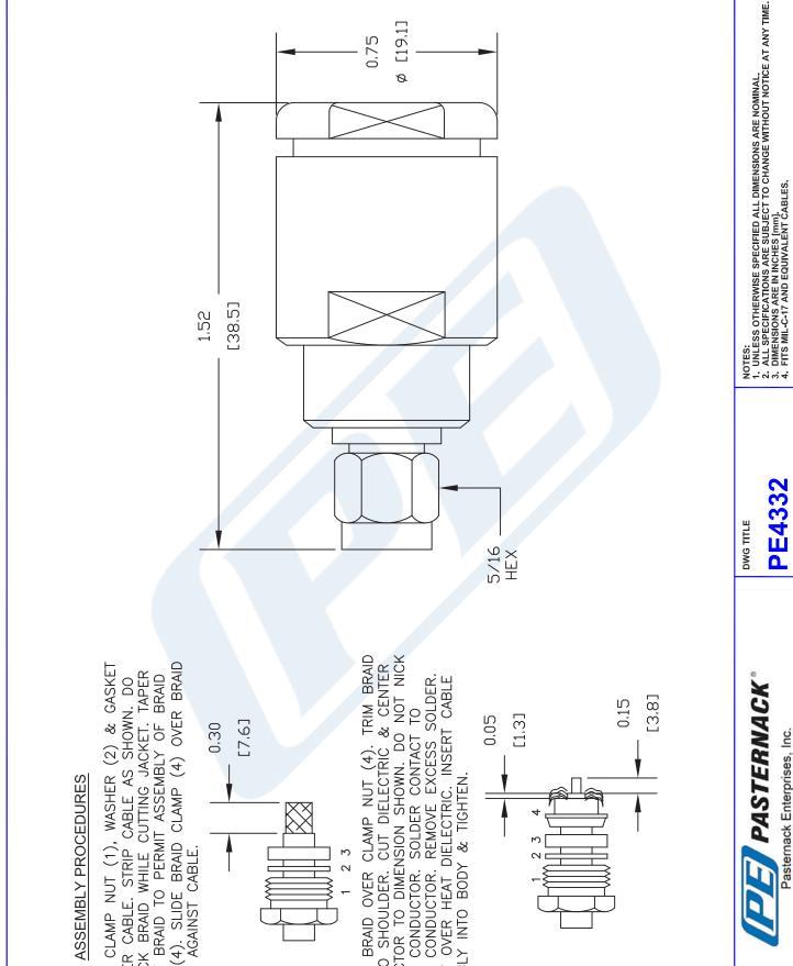
CONDUCTOR TO DIMENSION SHOWN. DO NOT NICK CLAMP NUT (4). TRIM BRAIL CUT DIELECTRIC & CENTER EXCESS SOLDER. DO NOT OVER HEAT DIELECTRIC. INSERT CABLE 0.05 [1,3] CENTER CONDUCTOR. SOLDER CONTACT ASSEMBLY INTO BODY & TIGHTEN. REMOVE BACK TO SHOULDER. 2. FORM BRAID OVER CONDUCTOR. CENTER
