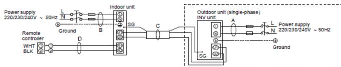
(SG : Shows the ground for the shielded cable.)
