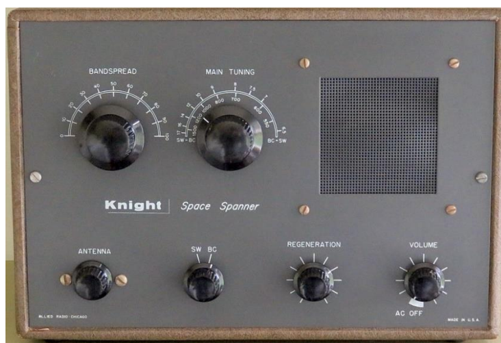
Model S-243 Allied Knight-Kit Space Spanner Short-Wave Receiver Tuned 6-17 MCS (MHz) Shortwave plus the Broadcast Band
