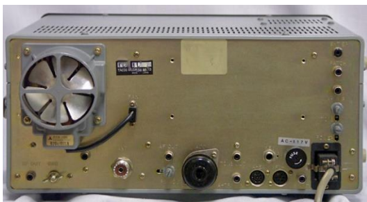
Rear Panel of the FT-101ZD Note Optional Fan is Installed See Tape over DC Module Connector 8 Note Power Connector at Lower Right W9MXQ
