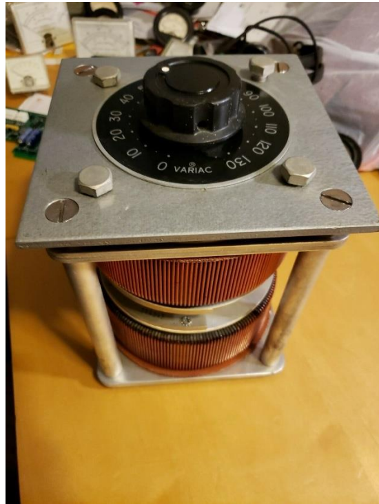
General Radio Dual W20G2 140-0-140 VAC Autotransformer Showing the two identical connection panels for the tandem 0-140 VAC autotransformers. Showing the top panel with the voltage control knob plus additional view of the mechanical construction.
