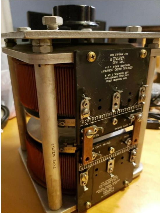
General Radio Dual W20G2 140-0-140 VAC Autotransformer Showing the two identical connection panels for the tandem 0-140 VAC autotransformers. Showing the top panel with the voltage control knob plus additional view of the mechanical construction.
