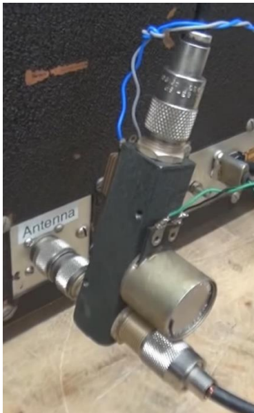
Dow Key Antenna Switching Relay See description, below, for notes about how this is connected. Mr. Carlson’s Lab© on YouTube™
