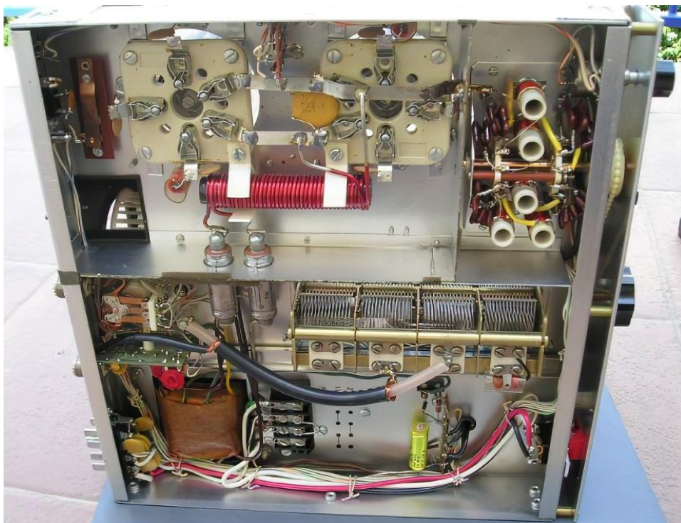
Drake L-4B Linear Amplifier – Bottom Interior View Front Panel to the Right
