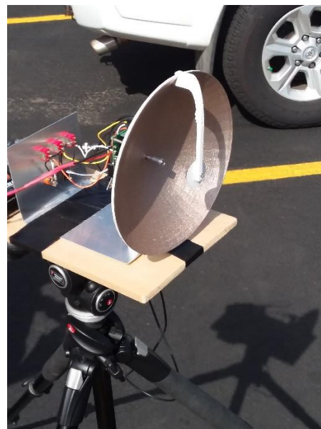
WF0T's 122 GHz rig. The dish is 3-D printed.
