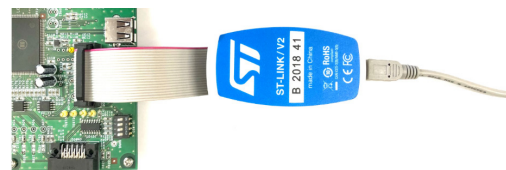
Figure 7. Debugger Connected with CN103
