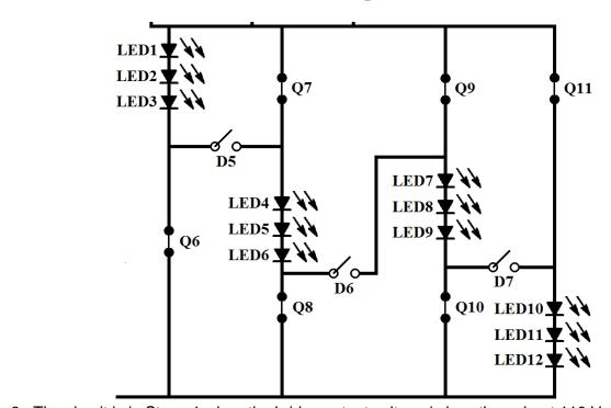
Figure 3: The circuit is in Stage 1 when the bridge output voltage is less than about 110 V. All four of the LED strings are in parallel in Stage 1.
