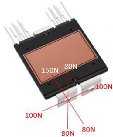
Figure 13. Force Limitations on the Power Terminal in All Axis
