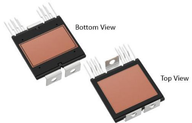
Figure 1. VE-Trac Dual Power Module Showing the Top and Bottom View
