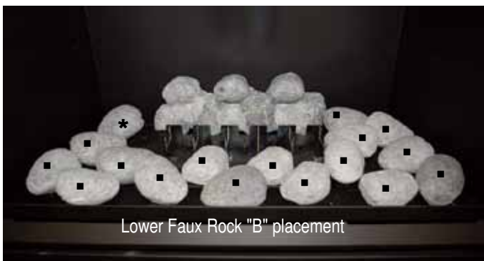
Figure 38c. Placement of (17) seventeen Lower "B" faux ceramic rocks. Note approximate location and placement. (Do not cover the burner holes if possible). (Place one of the rocks on top of the Pilot cover *).
