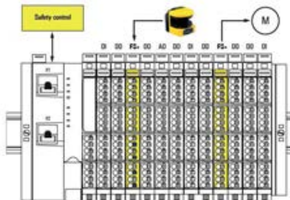
Example set-up of safe I/O modules (FS o ) in a u-remote station
