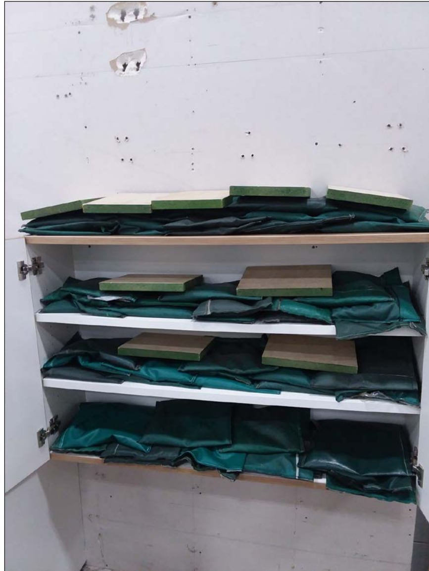
Wall Mounted Cabinet Load Test
