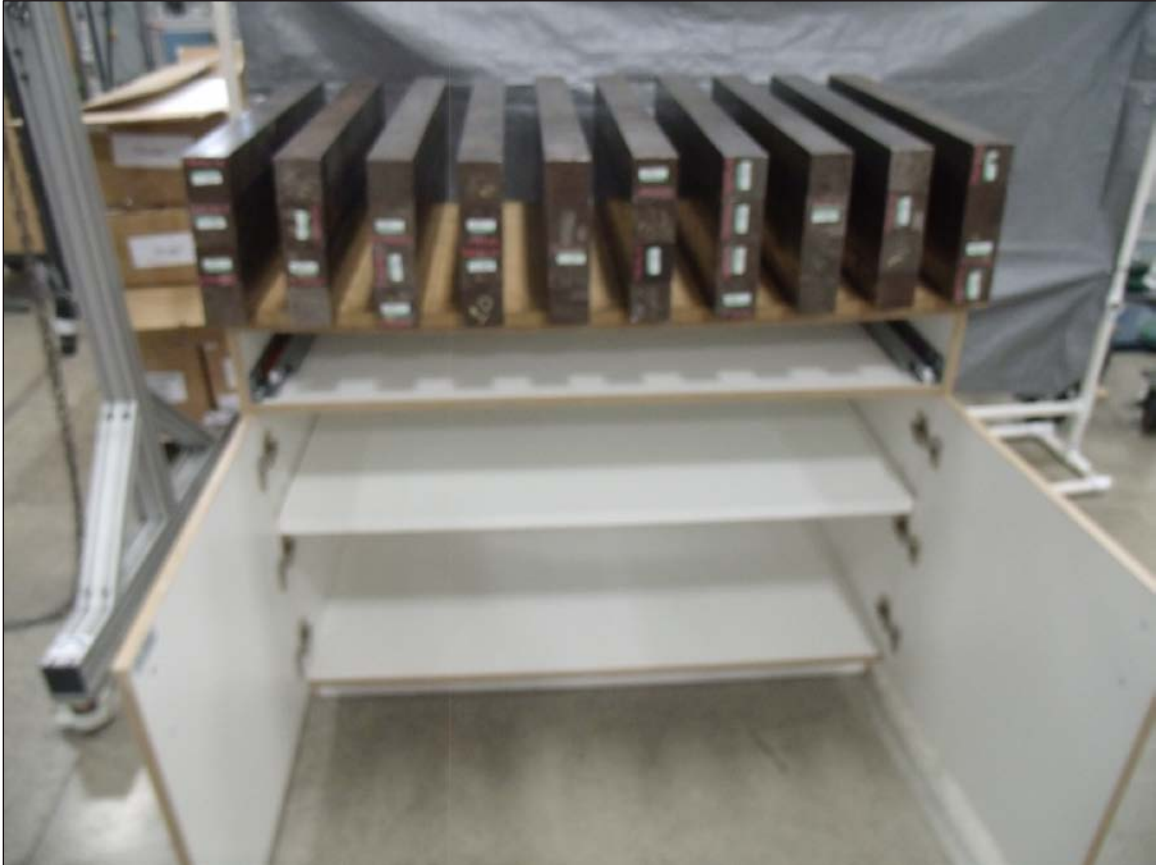
Cabinet Load Test
