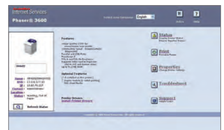
CentreWare IS helps administrators quickly install, configure, troubleshoot and analyse usage of the Phaser 3600 laser printer using any standard web browser.
