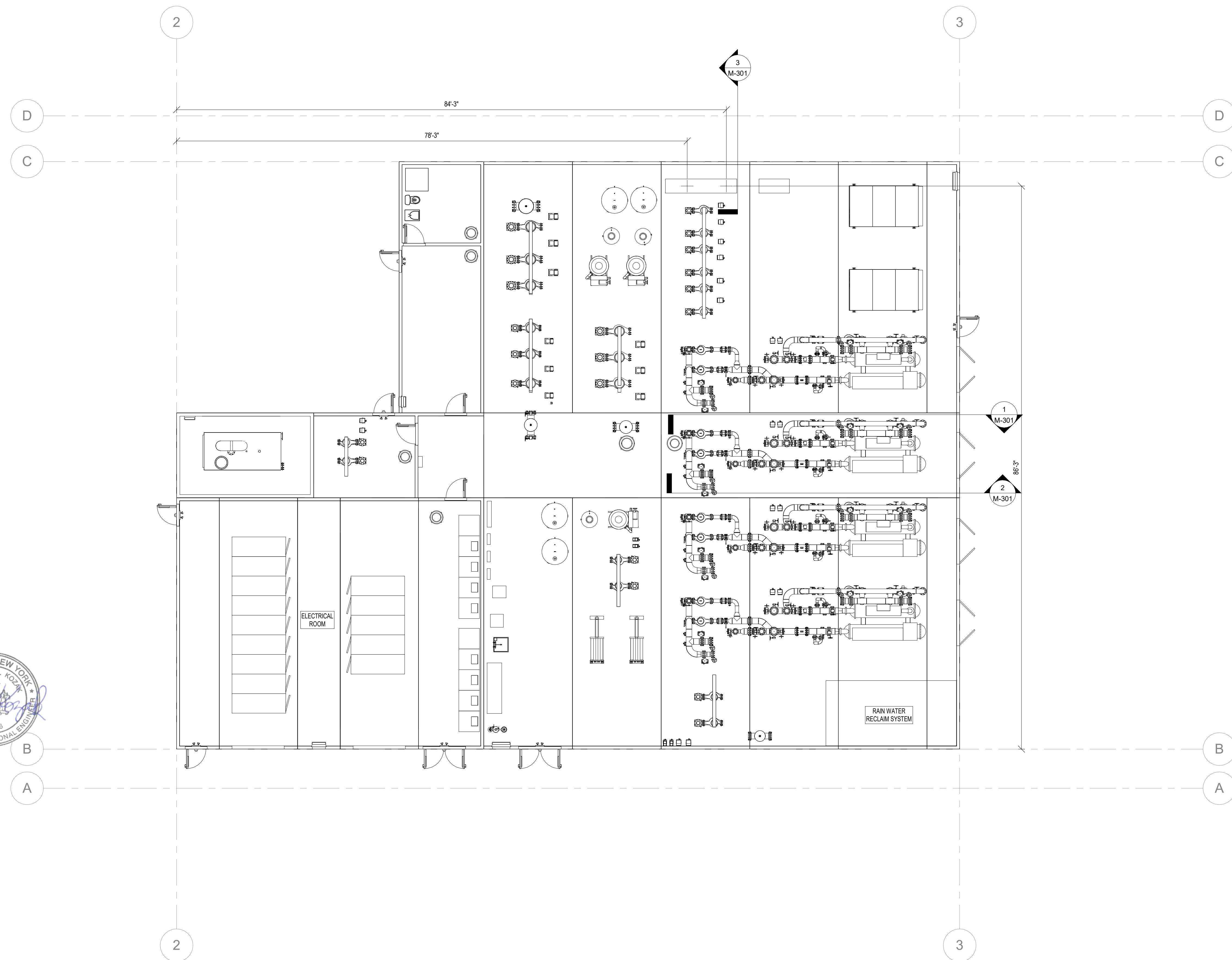
1 FIRST FLOOR - CHILLED WATER PIPING PLAN 1/8" = 1'-0" 0 4' 8' 16'
