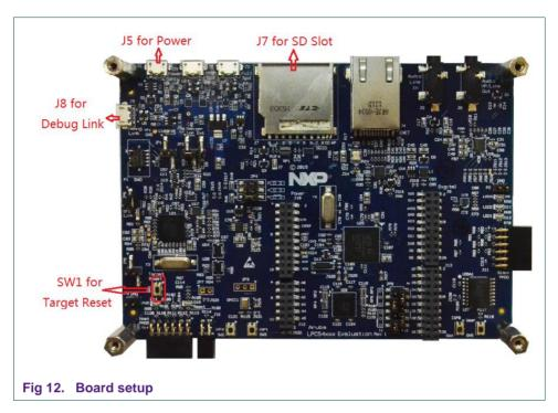
Plug SD card in J7 (SD slot) on the board. See Fig 12.
