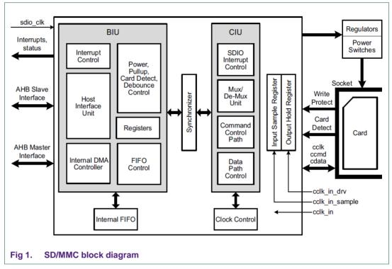
**Note:** The Card Detect and Write Protect signals are from the SD/MMC card socket, not the SD/MMC card itself.
