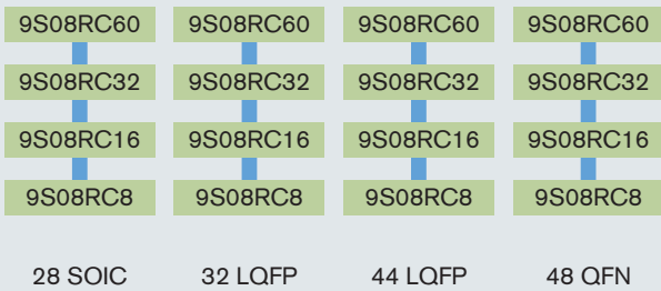
FIGURE 2. PACKAGE COMPATIBILITY IN MC9S08RC FAMILY
