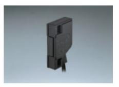
Applicable amplifiers: FX-100/300/311/410 series red LED type Sensing object: Liquid (Note) Applicable pipe diameter:  $\phi 8$  to  $\phi 80$  mm (transparent) (When using the attached tying bands) (including PFA translucent) Allowable bending radius: R10 mm or more Fiber cable length: 2 m (free-cut)
