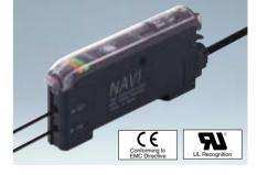
Sensing range (Red LED type): FT-B8 1,100 mm (LONG), 530 mm (STD), 180 mm (S-D) FD-B8 480 mm (LONG), 220 mm (STD), 75 mm (S-D) Supply voltage: 12 to 24 V DC ± 10 % Output: FX-311 □ NPN open-collector transistor FX-311 □ P PNP open-collector transistor Dimensions: W10  $\times$  H30.5  $\times$  D64.5 mm
