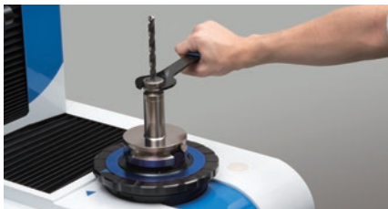
Tightening of a collet holder is possible. (Up to 60Nm) Move away the camera from the spindle when tightening.
