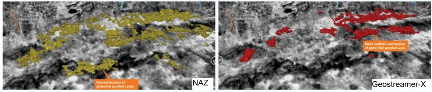
The NAZ seismic image is noisier, less coherent and potentially overpredicts the ponded sand distribution compared to PGS's multi-azimuth Geostreamer-X image
