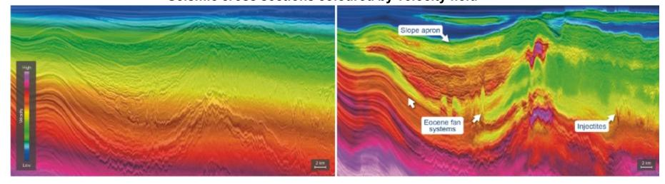
In this part of the west of Shetlands, an overburden of upper Tertiary extrusive volcanics benefited from a high-resolution FWI velocity model is beyond conventional tomographic techniques.
