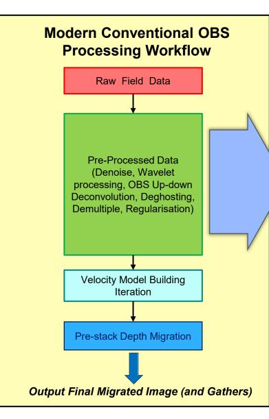
Processing has involved taking the original field data through a number of sequential stages each with parameters tested and chosen for a target. Across large regional surveys a single compromise parameter is usually chosen, meaning that future target specific reprocessing would often provide a better outcome, but compromised for a large survey. The end point product would be a migrated image in depth or stretched back to TWT.
