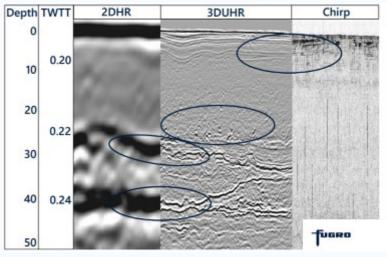
Comparative seismic techniques: resolution and depth of penetration
