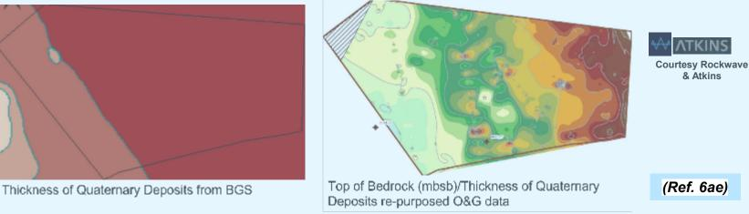
Legacy Oil and Gas seismic reprocessed and repurposed for shallow imaging
