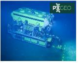
Usually, it take a long time to deploy nodes, but the regional hybrid survey (section 7.8c) deployed a combination of free drop and ROV pick up.
