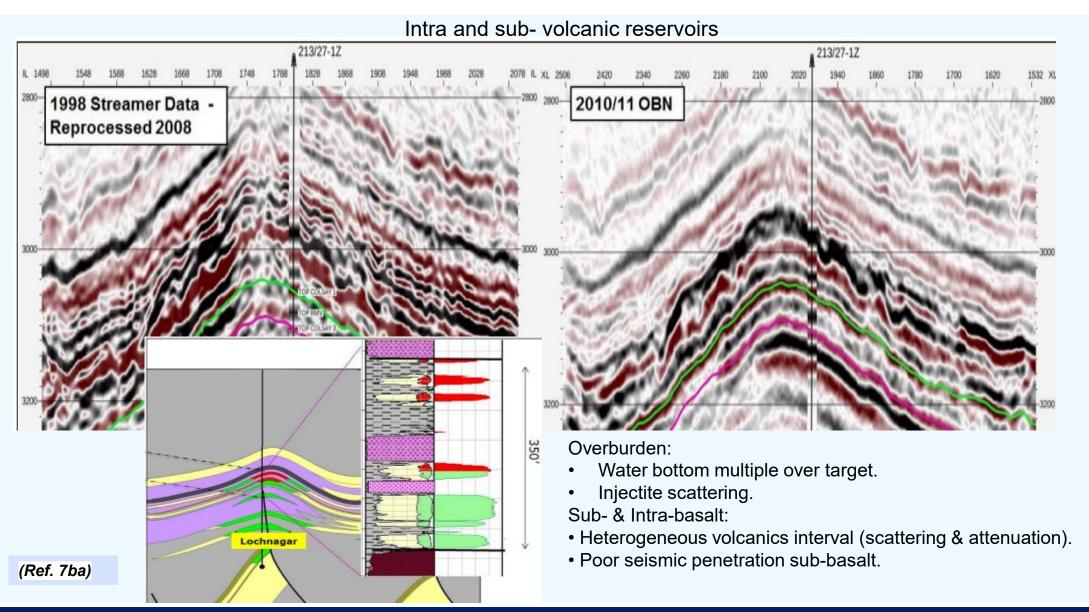
OBN: significant improvement in structural definition and velocity model. Individual basaltic flows and sand fairway confidence
