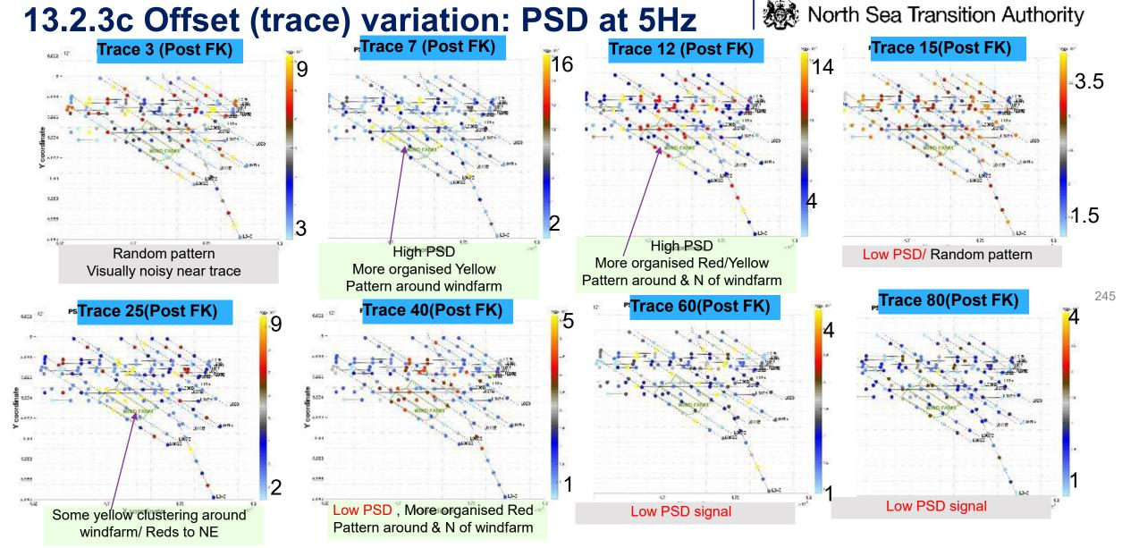
Observations: Low-mid offsets visually give best target signal to noise. Conclusions: 1) Near offsets residual primary/multiple contaminated and 2) Far offsets low signal to noise.
