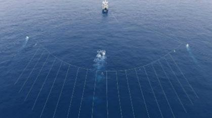
18x100m cables with tow width of ~200m
