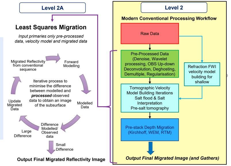
Both LS Migration FWI are iterative data driven processes that minimise the difference between modelled & observed data
