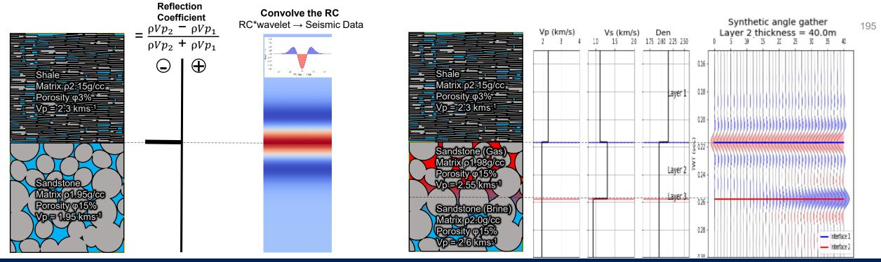
Factors influencing seismic response: Frequency bandwidth (wavelet pulse shape) controls the vertical resolution of detection.
