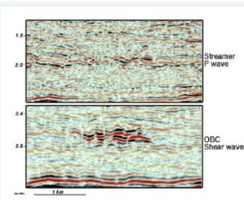
The reservoir can be clearly identified using shear wave data derived from the multi-component (OBC) seismic (see also section 5.6e)
