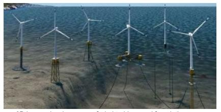
3D image showing range of wind turbines and foundations. Catenary cables & multiple anchor points, tension leg turbines OBN equipment fragile/ NOAR not laid over catenaries. AUV, ROV needed.
