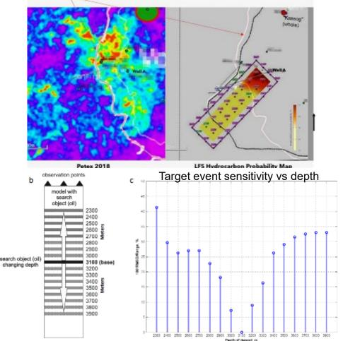
Modelling hydrocarbon scenarios indicates the oil water contact can be spatially detected by this technique. A further study then showed the degree of depth sensitivity between the modelled and observed OWC.
