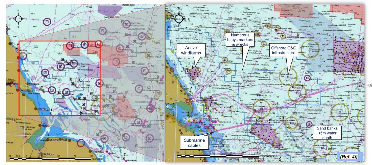
The SNS has a complex network of buoys and wrecks, existing O&G infrastructure (some of which could be re-used for CS purposes) active windfarms and those under development, along with associated cables and gas/potential CS pipelines.
