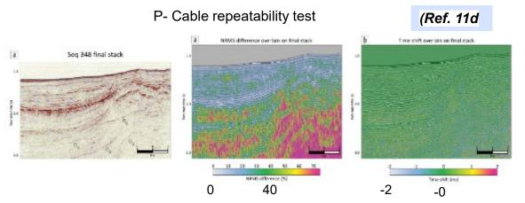
An inline from the final stack with water bottom multiples highlight by arrows (left) and the NRMS differences (middle) and small time shifts (right). The NRMS look acceptable for the shallow section but degrade quickly ~800m below mudline (compare with section 11.3). The time shifts are all small.
