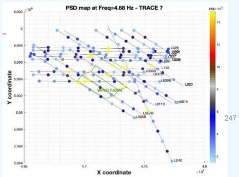
Slight increase in distribution of PSD magnitude discrete shot points around windfarm Low frequencies and near/mid offset
