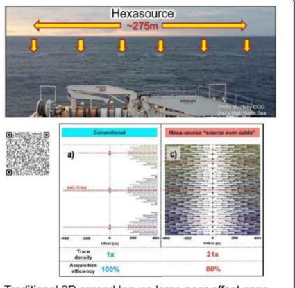
Traditional 3D spread leaves large near offset gaps which can be infilled with larger number of sources atop the cables.
