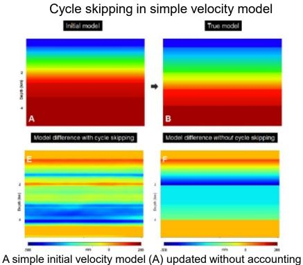
A simple initial velocity model (A) updated without accounting for cycle skipping creates a rapidly varying and erroneous model (E) compared to the true (B). 183
