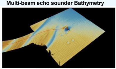
FIGURE 6: BATHYMETRY GRIDDED AT 0.2M RESOLUTION
