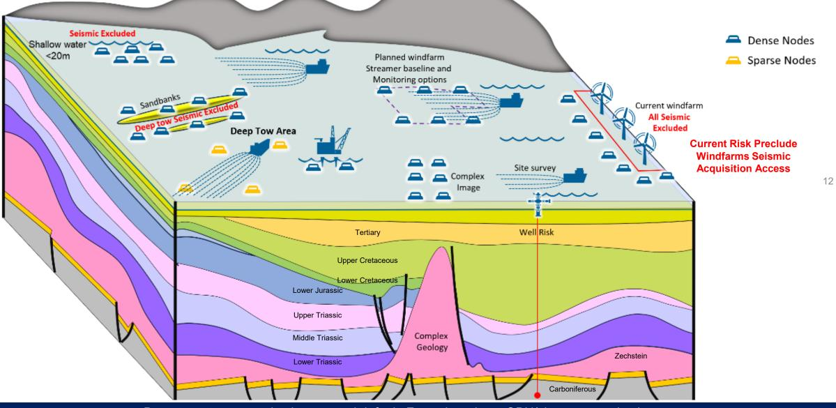
Deep tow streamer seismic expected default: Focus here is on OBN/site survey seismic
