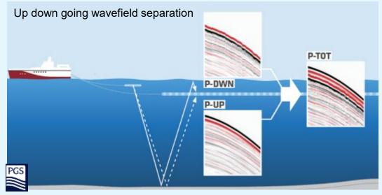
Multi-sensor streamer seismic transformed broadband seismic acquisition
