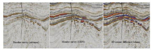
Commercially and operationally, it would be preferable to be able switch acquisition mode between baseline and monitors (streamer  $\leftrightarrow$  ocean bottom). In this case, switching from streamer to ocean bottom seismic creates very large discrepancies in seismic ray paths and very high levels of noise.
