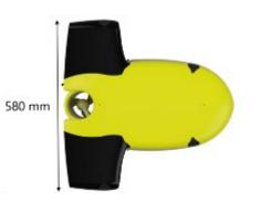
Largely automated node deployment, surveying and retrieval. The key advantages of 'Flying Nodes' are in the reduction in survey costs – expected to be less than half the cost of ROV deployed nodes, combined with excellent positioning accuracy and data quality. See also Section 7.20
