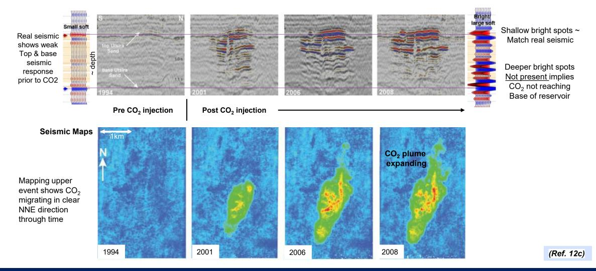
Proven CO<sub>2</sub> site: Linking prediction modelling to real CO2 sequestration
