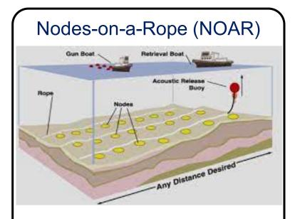
Nodes are anchored to a cable at a pre-defined spacing. Deployment and retrieval relatively simple and time efficient. This is the most frequently used technology. The cables hold sensors with no electronics in cable. A mature technology with >100 deployments worldwide.
