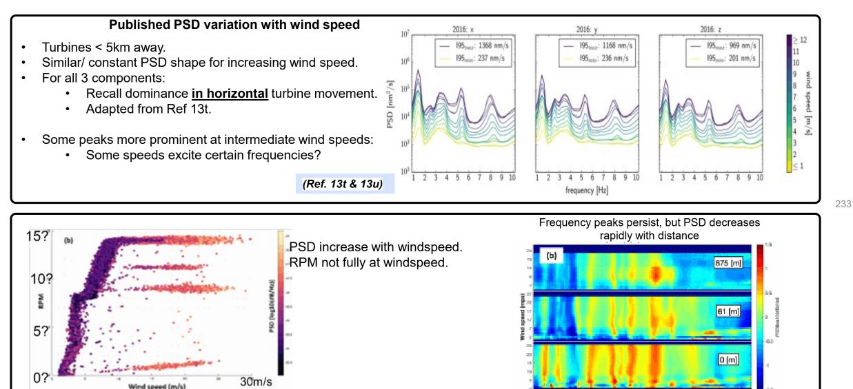
Discrete frequency peaks in PSD: Magnitude related to wind speed
