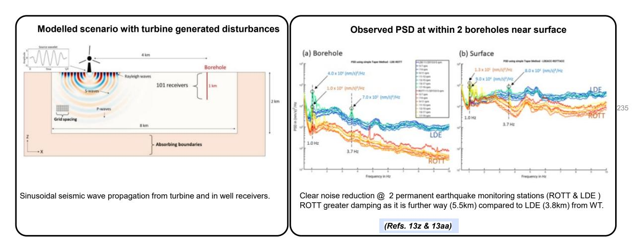
Turbines are detected at distance, but disturbance decreases with depth
