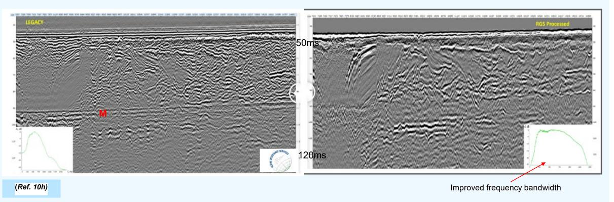
UHR reprocessing removing multiple and improving bandwidth
