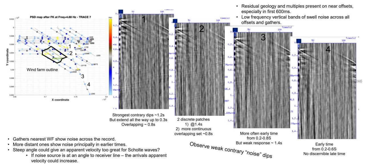
Example pre-stack gathers after FK filtering leaving the residual noise – potentially of windfarm origin
