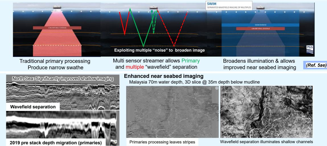
Extending seismic and improved near seabed imaging by multiple "noise". Works best in deep water.
