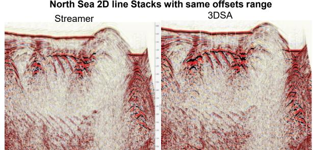
3DSA has similar frequency content and signal to noise to streamer 3DSA not affected by crossline strumming
