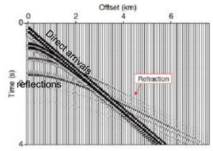
Refractions rely upon sound waves bending (refracting like prism) and can be observed on reflection seismic records
