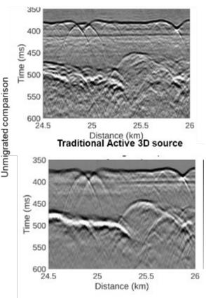
A deep water/ long offset 16 cable 3D streamer survey was acquired with and without active sources (i.e. just using vessel noise) and produces a passable low fidelity image of the gross structure of the top 300ms. This is frequency band limited up to 30Hz because of the long horizontal distances between vessel and receivers.
