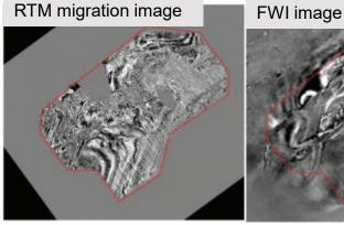
FWI fills acquisition holes and extended image from node coverage (red polygon) to shot coverage.
