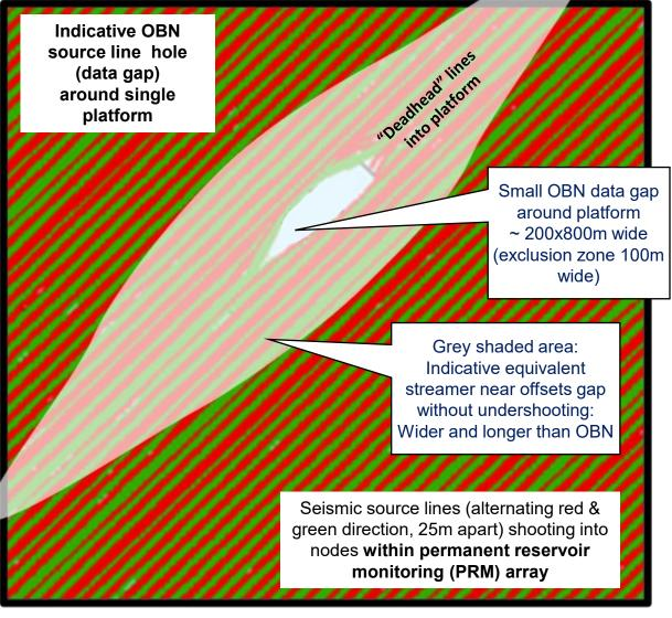
Indicative data gap between streamer and nodes around single obstruction
