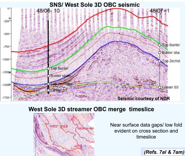
Very limited near offset data is apparent even on <u>HD</u> OBN surveys (Golden Eagle 7.4). Seabed can be imaged with very dense (and expensive) <u>UHD</u> OBN and seismic imaging technologies (section 6.10 & 7.12).
