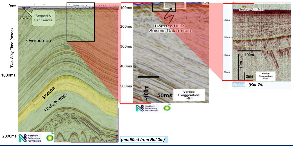
SNS storage complex elements and a comparison of imaging resolution between reservoir HR and windfarm seismic
