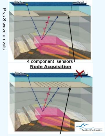
4C sensors: (3 geophones (x,y,z) – also MEMS or optical for OBC + 1 hydrophone Often 2<sup>nd</sup> vessel needed for node deployment and retrieval
