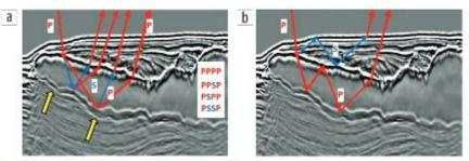
Figure 1. (a) Four different arrivals for a single incident P-wave to the top of salt raypaths of some mode-converted reflections at the salt boundaries. (b) Raypaths of interbed multiples between salt boundaries and water bottom.
