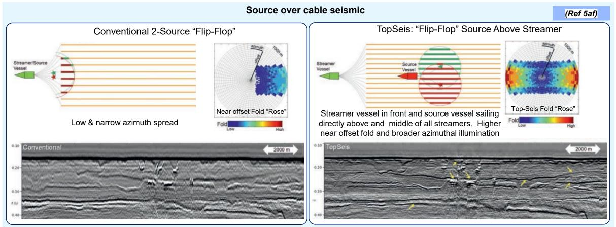
Complex shallow geological comparison with post-glacial Neogene channels several gas water bottom pockmarks. Both images show shallow structures, but TopSeis provides better definition.
