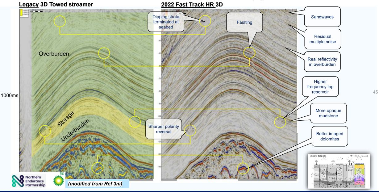
SNS storage complex elements and a comparison of improvements via modern HR seismic acquisition
