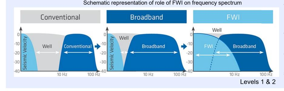
"Level 3" FWI processing can be undertaken to 100Hz, so the FWI image becomes the product and there is no need to combine with the real data. However, the result may be model driven (section 10.17) and represents pseudo-velocity rather than the velocity\*density product of a conventional seismic image.
