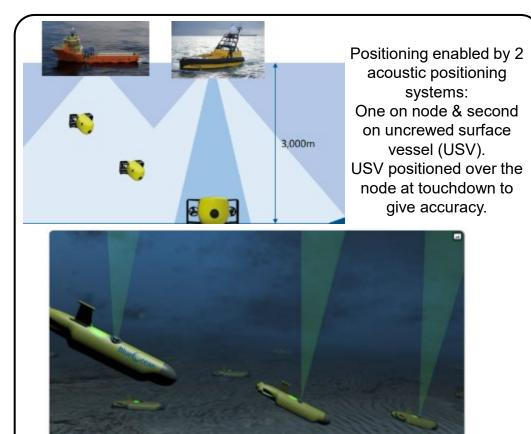
Fleets of autonomous, self-positioning subsea nodes could soon be acquiring ocean bottom seismic data
