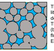
The porosity space will vary with lithology (mineralogical parameters), depth & age of the rock. The porosity is filled with fluid – water (brine), oil, condensate, gas, or injected fluids such as  $CO_2$ . Each fluid type varies in characteristics:
