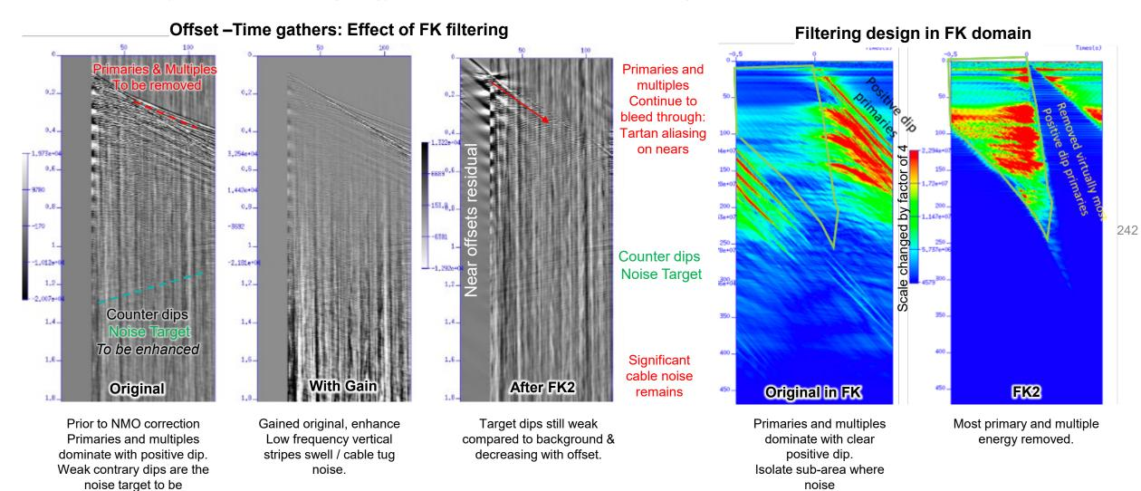
FK filtering leaves target dips at limit of detection and weak residual primaries/ multiples
