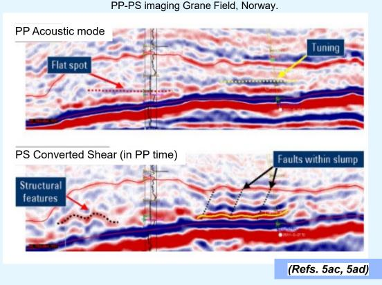
PP: both geological and fluid information; PS: better definition of the sand body geometry (internal deformation features, structure, and sand injections)
