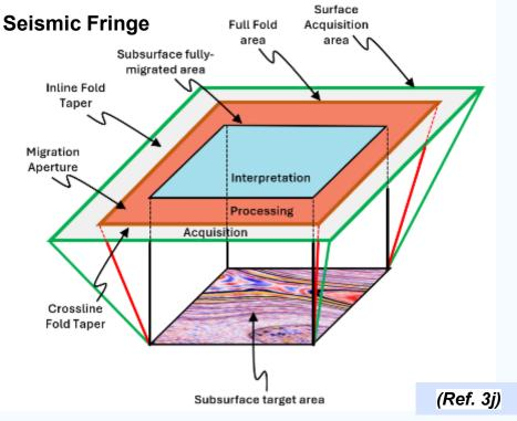
Seismic acquisition footprints much large than target area
