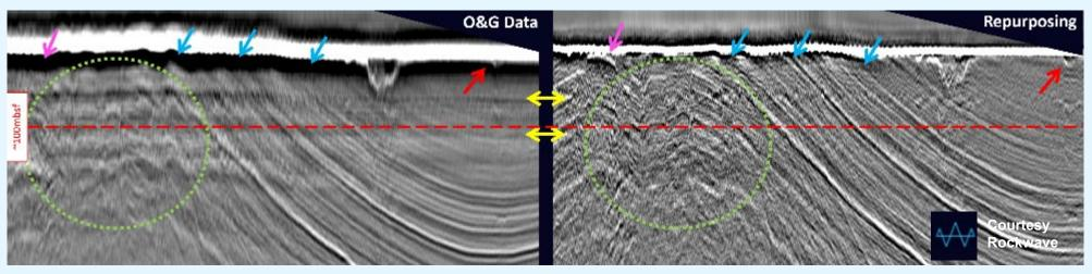
Reservoir seismic reprocessed for shallow imaging: Celtic Sea
