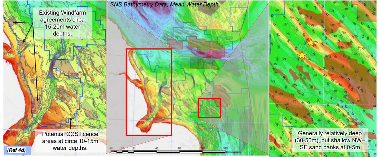
SNS water depth bathymetry can be beyond the limits of deep tow seismic
