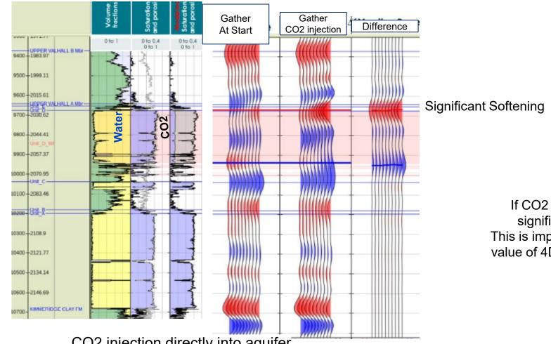
If CO2 migrates into aquifer, then a significant response is expected. This is important, as it shows the potential value of 4D even within a depleted oil/gas field.
