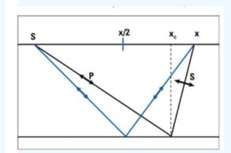
PP reflection point can be determined geometrically, PS depends upon the medium parameters
