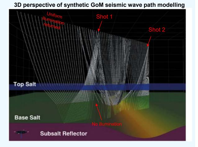
2 Simulated shots and resulting distorted reflection ray paths as (2) traverses more complex high velocity salt
