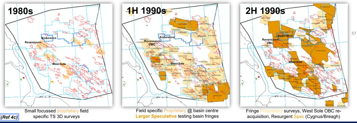
Early growth of 3D seismic, significant increase in coverage through early 1990s
