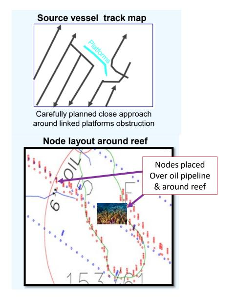
Carefully planned seabed seismic can be undertaken around very many obstructions and sensitive areas
