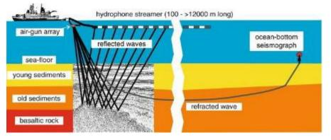
Refraction means that not all the subsurface is equally or evenly imaged. This is a particular problem where there is complex subsurface geometries and rocks with significantly different acoustic properties against each other e.g., SNS contains carbonates and evaporites with large velocity contrasts to shales and sandstones, with structures dominated by complex salt movement histories.
