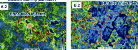
High resolution FWI and machine learning velocity models can be used to characterise the potential fluid fill of injectites
