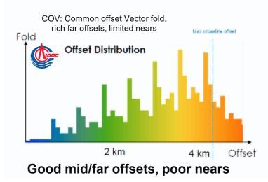
OBN seismic parameters limited near offset, excellent mid & far offset fold
