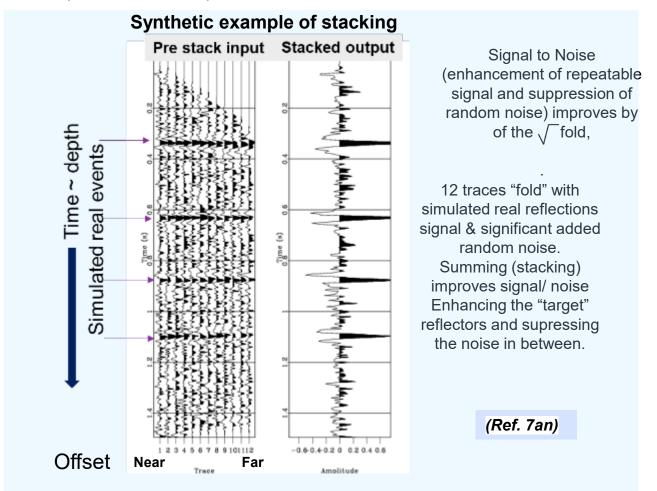
Stacking several traces from the same subsurface point (fold) directly reduces the background noise and enhances geological signal
