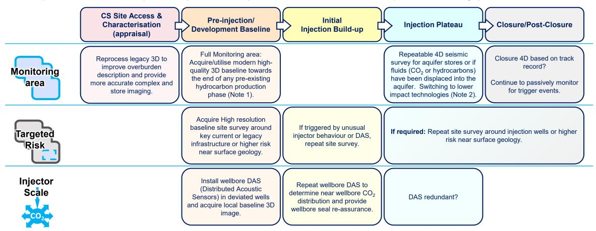
Note 1) predominantly streamer but consider benefit of incorporating a) sparse nodes to provide a comprehensive velocity field for deeper targets b) optional localised HD node patches around surface infrastructure for hybrid imaging.
