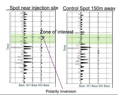
More recently (2023- section 12.10b) Spotlight has been trialled on the Project Greensand CCS test area in Denmark. This involved a baseline and 2 monitor surveys using 25 nodes deployed throughout and 80 shots at 7 stationary locations. The shots typically achieving 1m repeatability.
