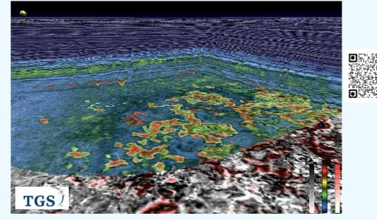
Predicted velocity model using machine learning (EarthNET)
