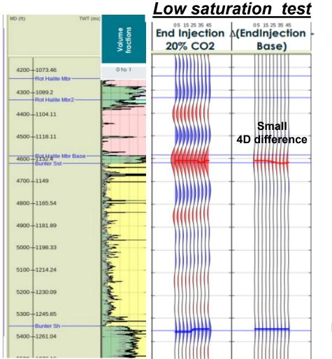
Partial (20%) CO2 Saturation at limits of detection Smaller effect because of heterogenous fluid mixing model
