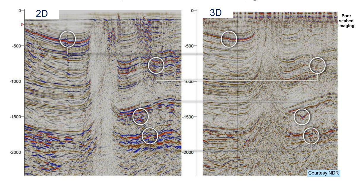
3D seismic offers significant imaging improvements over 2D seismic data, but struggles with salt diapirism
