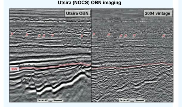
Building on earlier injectite experience (e.g., Alba – section 5.6d& 5.6e), fine scale imaging has been provided in the regional Utsira HDOBN survey. OBN illuminated from all sides and sampled up to 25 times better than with a narrow azimuth streamer 3D.
