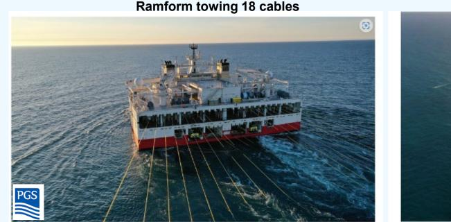
Ramform Hyperion towing 18 x 75m x 8 025m GeoStreamer spread.
