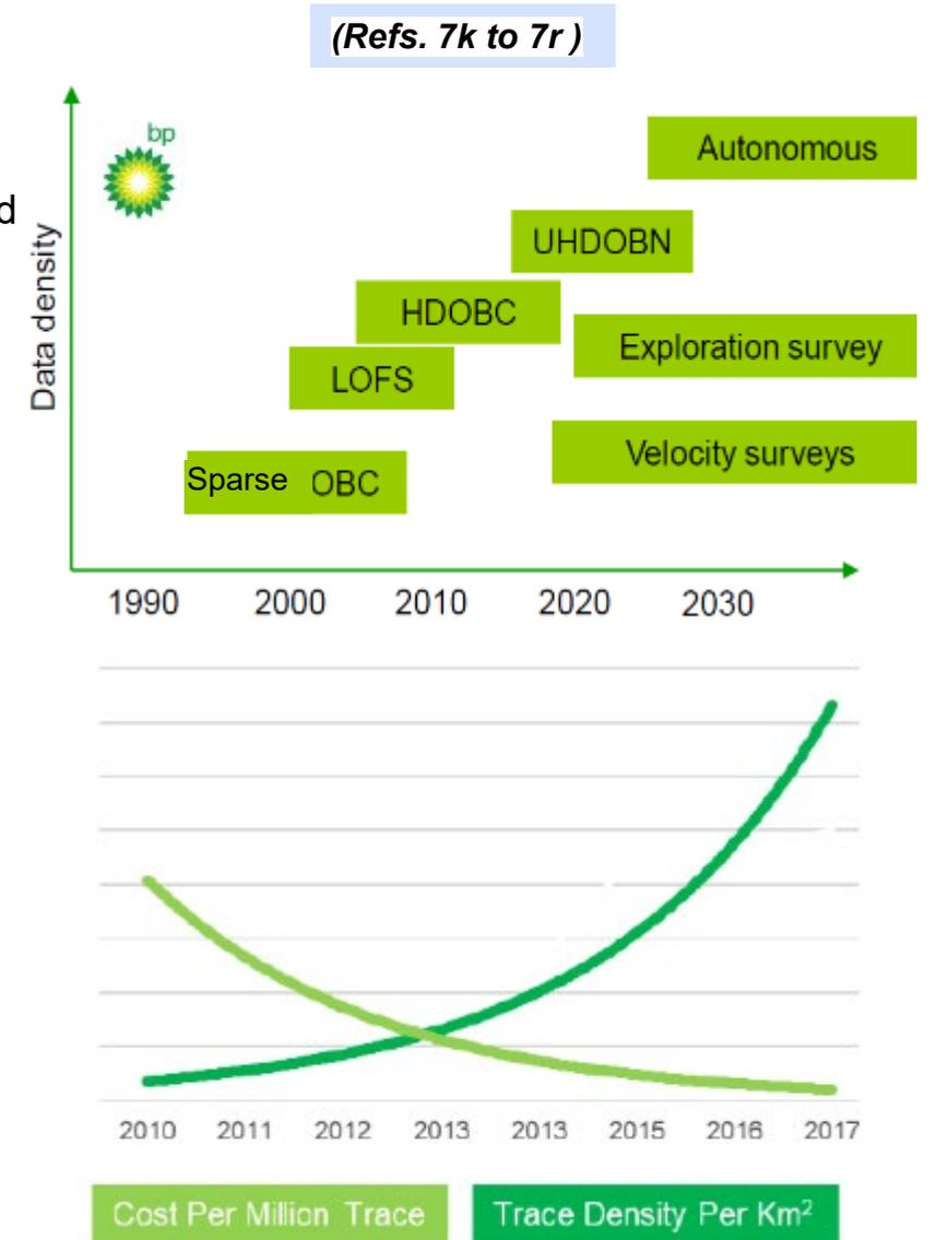
Whilst trace densities have been significantly increasing, the cost per million traces has provided a dramatic fall (computing power increase being a notable contributor).
