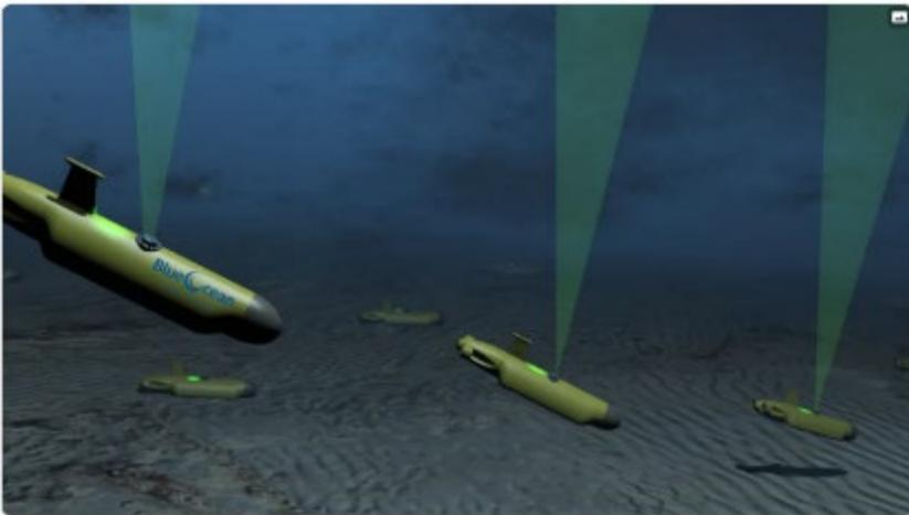
Fleets of autonomous, self-positioning subsea nodes could soon be acquiring ocean bottom seismic data
