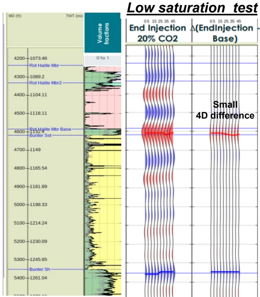
Partial (20%) CO2 Saturation at limits of detection
