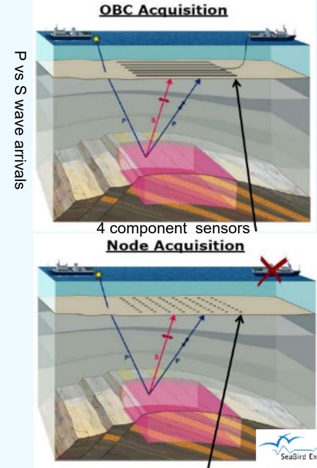
4C sensors: (3 geophones (x,y,z) – also MEMS or optical for OBC + 1 hydrophone
