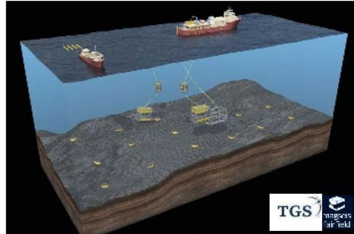
Nodes are deployed by ROV across seabed. Allows some flexibility in deployment pattern, especially if working close to existing infrastructure.
