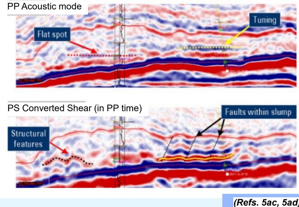
PP: both geological and fluid information; PS: better definition of the sand body geometry ( internal deformation features, structure, and sand injections)
