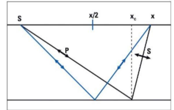
PP reflection point can be determined geometrically, PS depends upon the medium parameters
