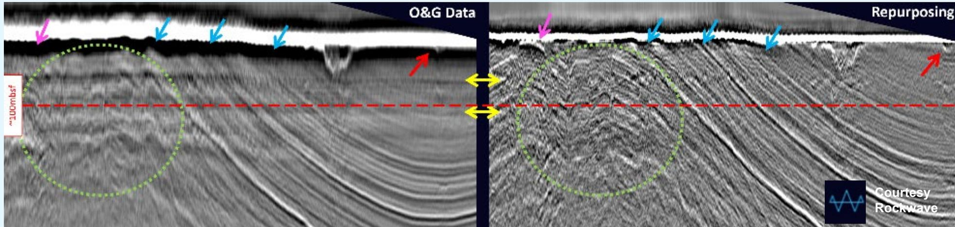
Reservoir seismic reprocessed for shallow imaging: Celtic Sea
