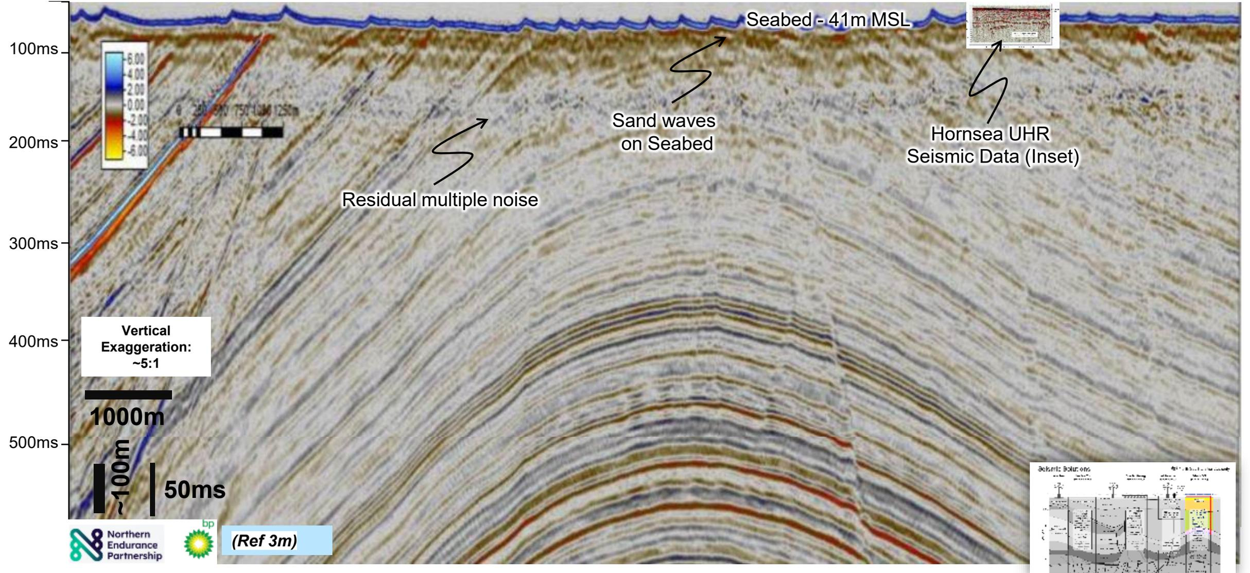
Windfarm / geotechnical seismic results completely different level of definition
