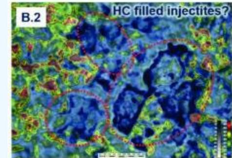
High resolution FWI and machine learning velocity models can be used to characterise the potential fluid fill of injectites
