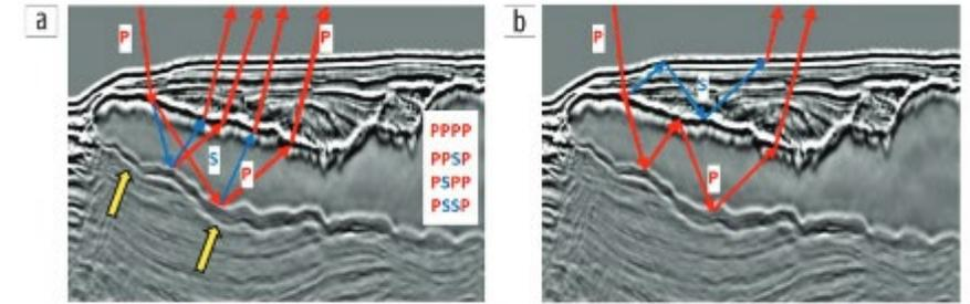
Figure 1. (a) Four different arrivals for a single incident P-wave to the top of salt raypaths of some mode-converted reflections at the salt boundaries. (b) Raypaths of interbed multiples between salt boundaries and water bottom.
