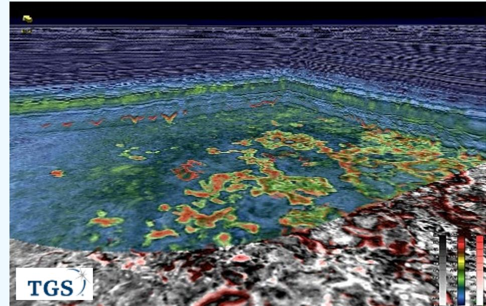
Building on earlier injectite experience (e.g., Alba – section 5.6d & 5.6e), fine scale imaging has been provided in the regional Utsira HDOBN survey. OBN illuminated from all sides and sampled up to 25 times better than with a narrow azimuth streamer 3D.
