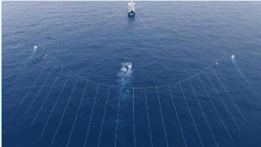
18x100m cables with tow width of ~200m
