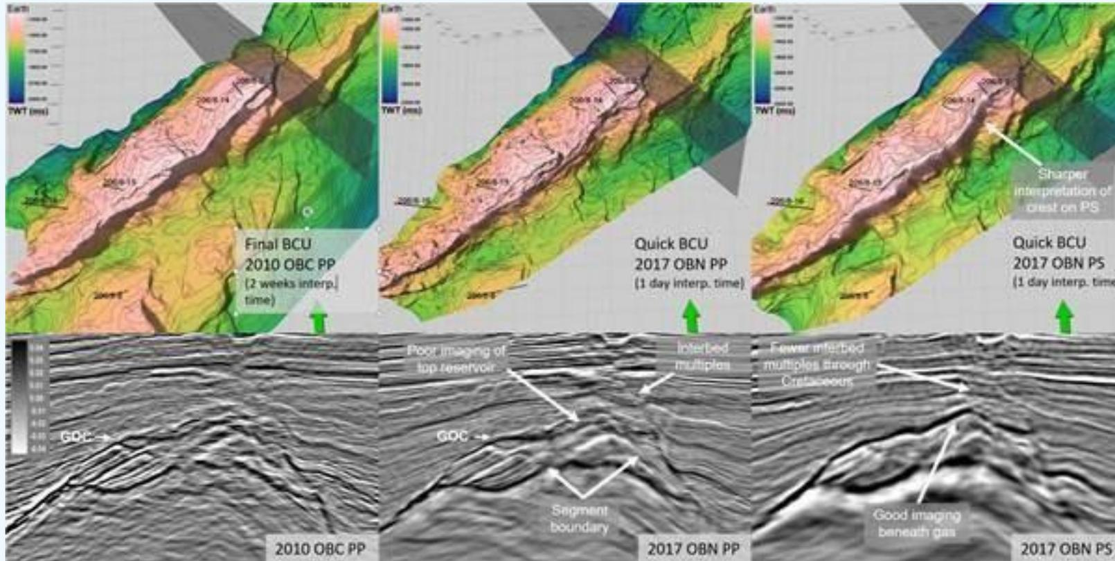
This comparison builds on Clair HDOBN imaging description (section 7.12) differences in both cross section and Base Cretaceous Unconformity (BCU) mapping.
