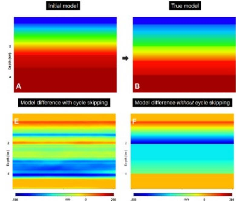
A simple initial velocity model (A) updated without accounting for cycle skipping creates a rapidly varying and erroneous model (E) compared to the true (B).
