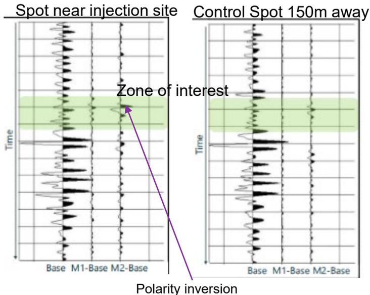
More recently (2023- section 12.10b) Spotlight has been trialled on the Project Greensand CCS test area in Denmark. This involved a baseline and 2 monitor surveys using 25 nodes deployed throughout and 80 shots at 7 stationary locations. The shots typically achieving 1m repeatability.
