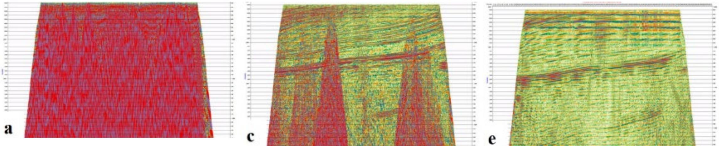
Results of the de-noising sequence a) the input Z data, c) after FX in cross-line direction and e) the hydrophone data used as reference for the directional filtering. (Deschizeaux (2013) EAGE).
