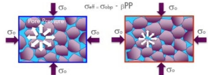
Gas reservoir depletion -> increases effective stress and stiffens the rock matrix -> Measurable increase in velocity. Physical compaction is insignificant
