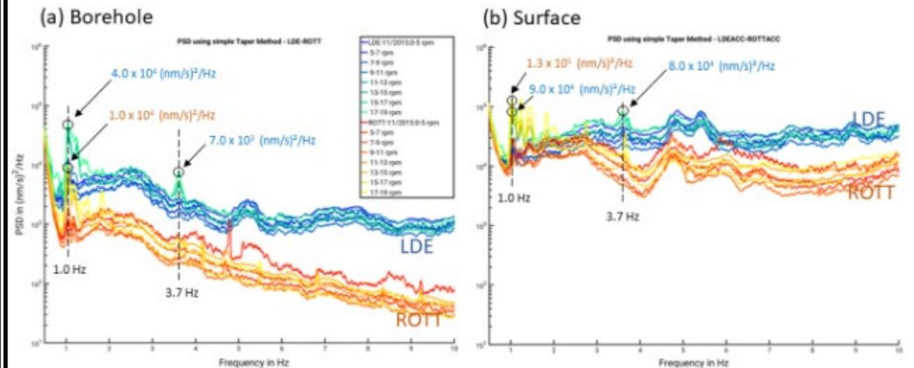
Clear noise reduction @ 2 permanent earthquake monitoring stations (ROTT & LDE )
