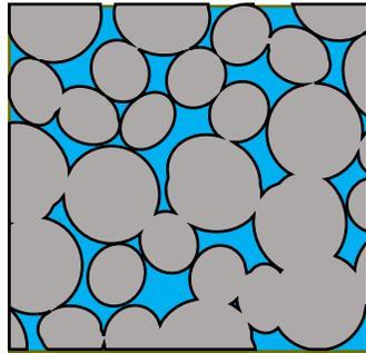
The porosity space will vary with lithology (mineralogical parameters), depth & age of the rock. The porosity is filled with fluid – water (brine), oil, condensate, gas, or injected fluids such as CO<sub>2</sub>. Each fluid type varies in characteristics:
