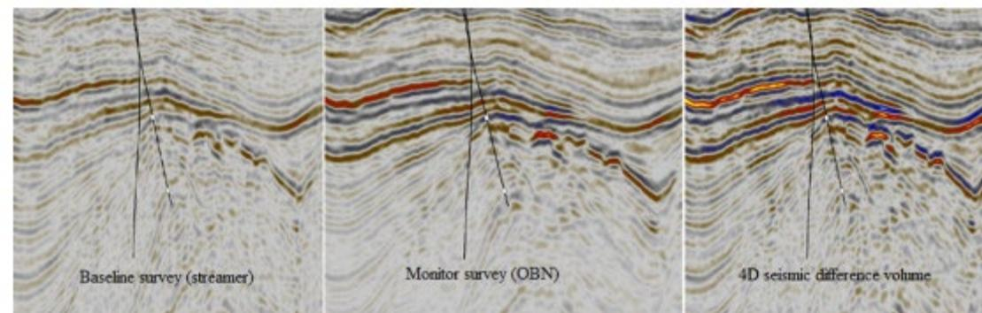
Commercially and operationally, it would be preferable to be able switch acquisition mode between baseline and monitors (streamer ↔ ocean bottom). In this case, switching from streamer to ocean bottom seismic creates very large discrepancies in seismic ray paths and very high levels of noise.
