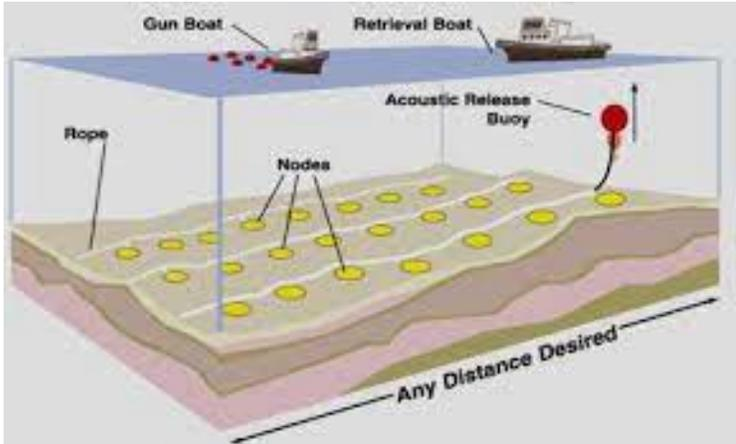
Nodes are anchored to a cable at a pre-defined spacing. Deployment and retrieval relatively simple and time efficient. This is the most frequently used technology. The cables hold sensors with no electronics in cable. A mature technology with >100 deployments worldwide.
