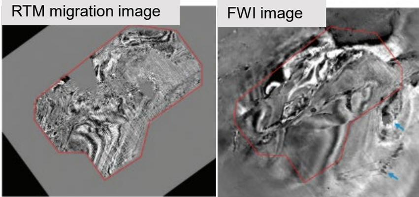
FWI fills acquisition holes and extended image from node coverage (red polygon) to shot coverage.
