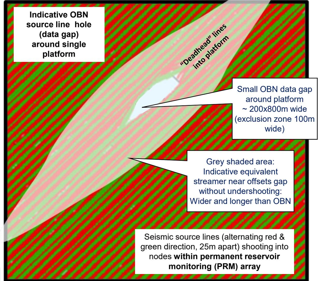
A seismic streamer data gap is significantly larger data hole than OBN
