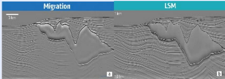
Standard PSDM gives uneven illumination. LSM balances the amplitudes, reduces shadow zones and improves temporal resolution (bandwidth).
