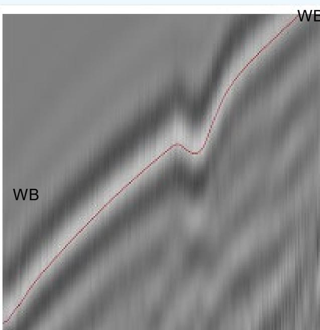
Water bottom tracks along strong trough, with balanced sidelobe peaks either side
