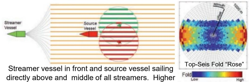
Streamer vessel in front and source vessel sailing directly above and middle of all streamers. Higher near offset fold and broader azimuthal illumination
