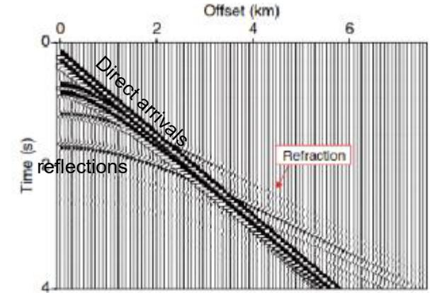
Refractions rely upon sound waves bending (refracting like prism) and can be observed on reflection seismic records
