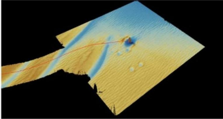
FIGURE 6: BATHYMETRY GRIDDED AT 0.2M RESOLUTION
