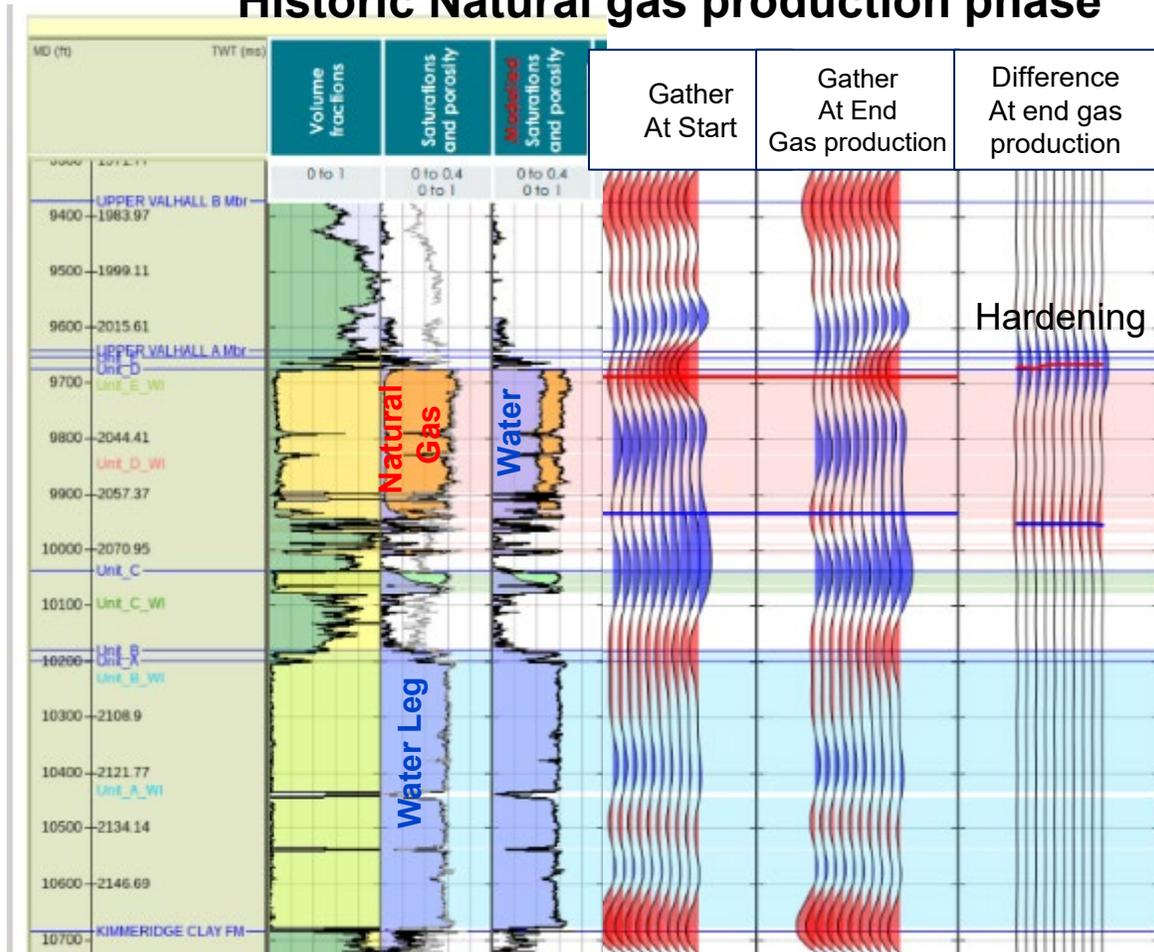
As a depleted field Gassmann fluid substitution is required to remove residual HC's prior to calculations for effects of CO<sub>2</sub> injection. Post historic gas production the seismic response is expected to have hardened (depletion and some water influx).
