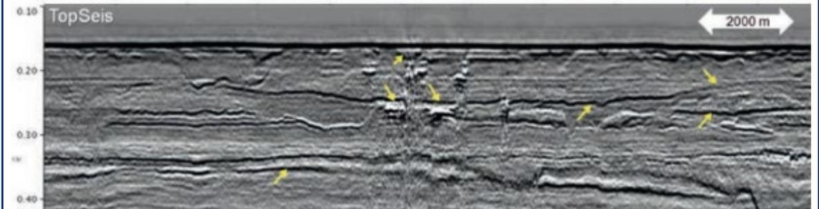
Complex shallow geological comparison with post-glacial Neogene channels several gas water bottom pockmarks. Both images show shallow structures, but TopSeis provides better definition.
