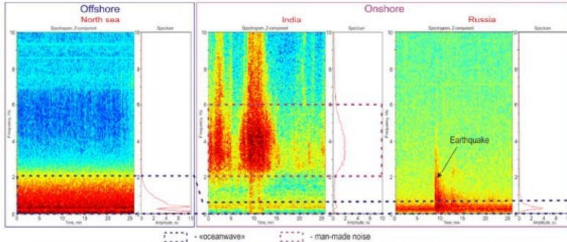
Figure 2: An example of an offshore and onshore passive seismic signal
