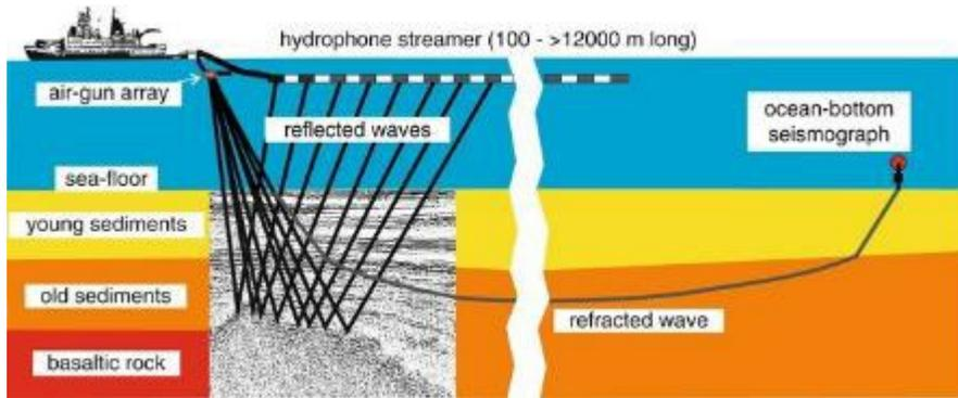
Refraction means that not all the subsurface is equally or evenly imaged. This is a particular problem where there is complex subsurface geometries and rocks with significantly different acoustic properties against each other e.g., SNS contains carbonates and evaporites with large velocity contrasts to shales and sandstones, with structures dominated by complex salt movement histories.
