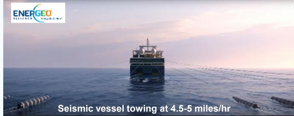
Seismic vessel towing at 4.5-5 miles/hr
