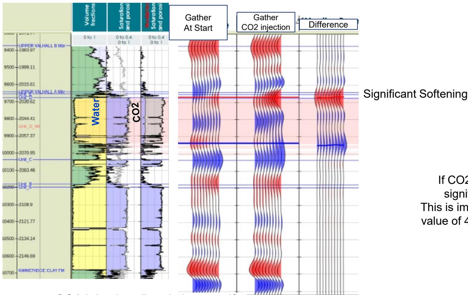
If CO<sub>2</sub> migrates into aquifer, then a significant response is expected. This is important, as it shows the potential value of 4D even within a depleted oil/gas field.
