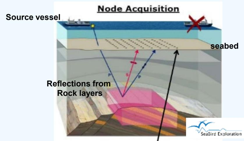
4 Component Pressure (hydrophone) and movement (x,y,z geophone) sensors
