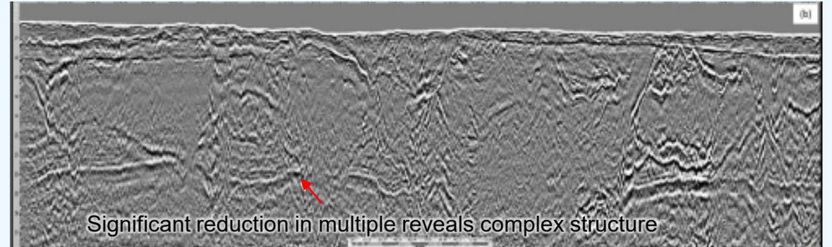
Like deep seismic, multi-channel processing of UHR seismic can greatly reduce noise (M multiple) & enhance signal.
