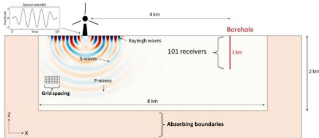
Sinusoidal seismic wave propagation from turbine and in well receivers.
