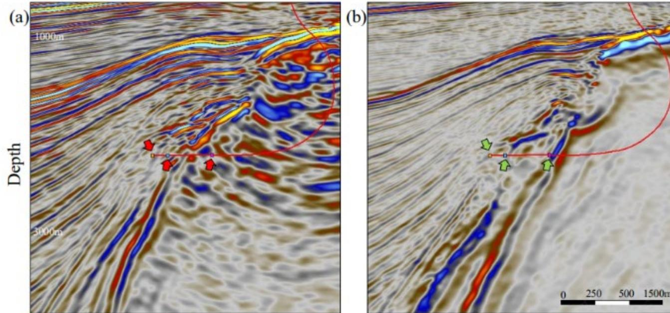
Salt diapir flank imaging with (a) legacy and (b) final velocity models overlaid with salt exit and horizon markers. Horizontal mis-ties at the reservoir level are greatly reduced with the updated velocity model.
