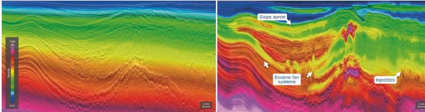
In this part of the west of Shetlands, an overburden of upper Tertiary extrusive volcanics benefited from a high-resolution FWI velocity model is beyond conventional tomographic techniques.
