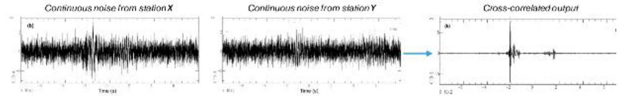
▶ If this noise is random, the only common "signal" is a function of the impulse response between the two stations
