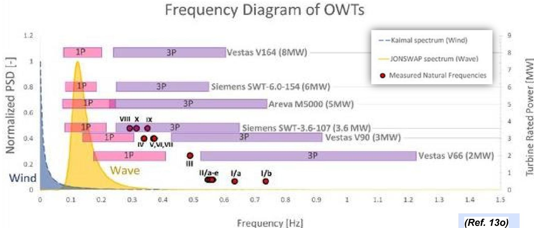
**Turbine loading generates discrete peaks in frequency spectrum**
