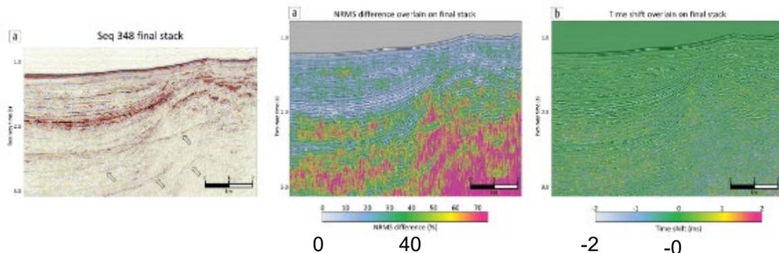
An inline from the final stack with water bottom multiples highlight by arrows (left) and the NRMS differences (middle) and small time shifts (right). The NRMS look acceptable for the shallow section but degrade quickly ~800m below mudline (compare with section 11.3). The time shifts are all small.
