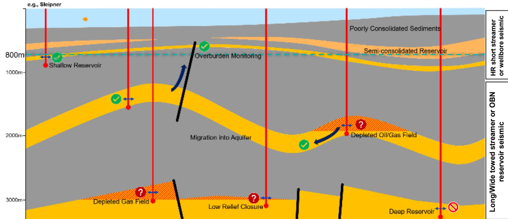
Detection of an amplitude change where CO<sub>2</sub> is injected into a pre-existing depleted natural gas field appears difficult and may require either:
