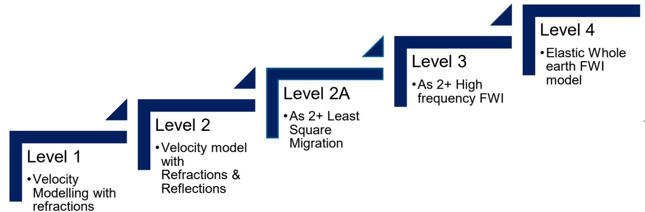
However, FWI is a highly nonlinear, iterative process whose success depends on the seamless addition of wavelength features that are missing from the starting velocity model. In order to resolve features that lie below the deepest turning point of the recorded refractions and diving waves, analysis depends upon the low frequency content of pre-critical reflections.
