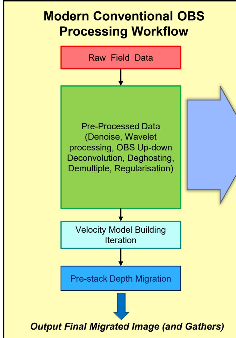
Processing has involved taking the original field data through a number of sequential stages each with parameters tested and chosen for a target. Across large regional surveys a single compromise parameter is usually chosen, meaning that future target specific reprocessing would often provide a better outcome, but compromised for a large survey. The end point product would be a migrated image in depth or stretched back to TWT.
