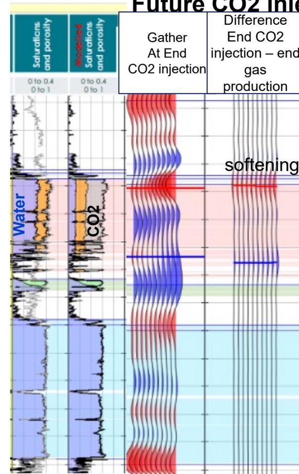
At the end of injection, the reservoir composition will be 50% CO<sub>2</sub>, 30% Natural gas, 20% Brine. Injection drives a pressure response but results in negligible difference in gather 4D residuals.
