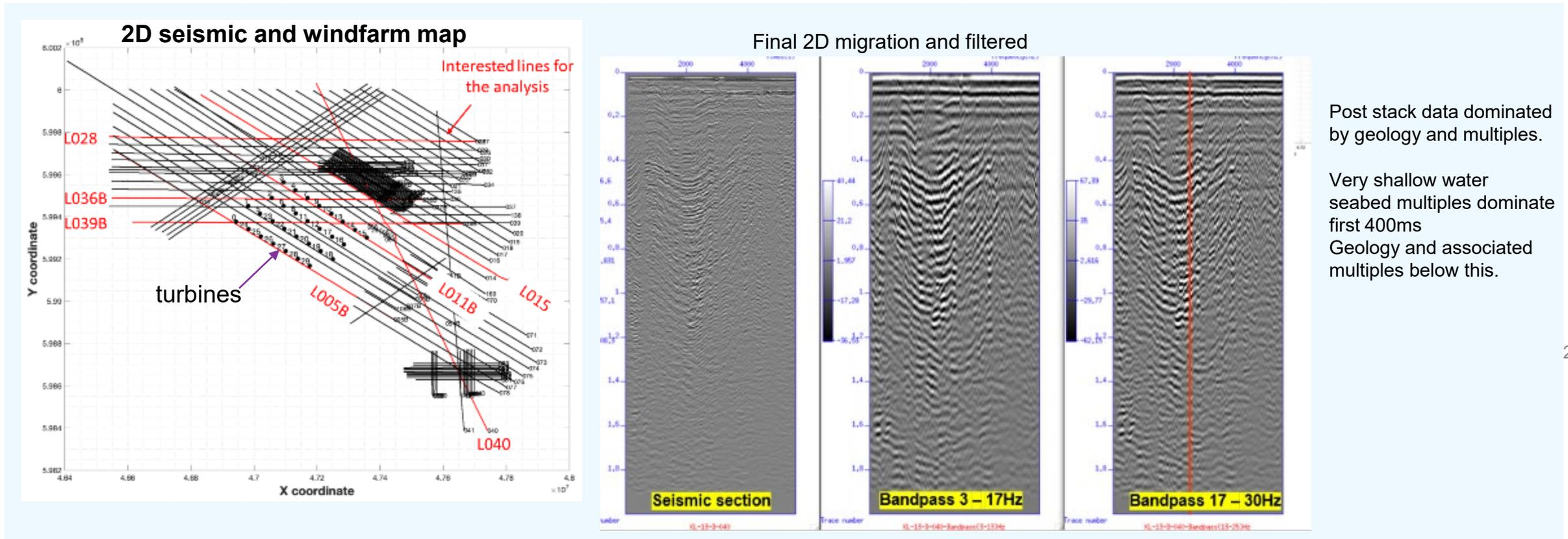
2D HR seismic survey comprised series of lines running E-W and NE-SW around and within a 30-turbine windfarm.
