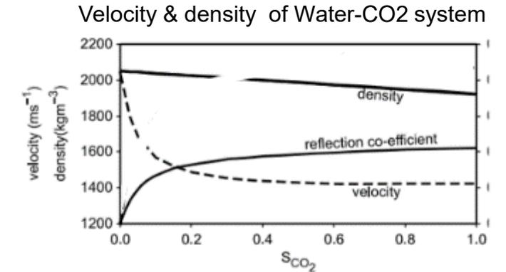
Large drop in seismic velocity for Small initial changes in CO<sub>2</sub> saturation
