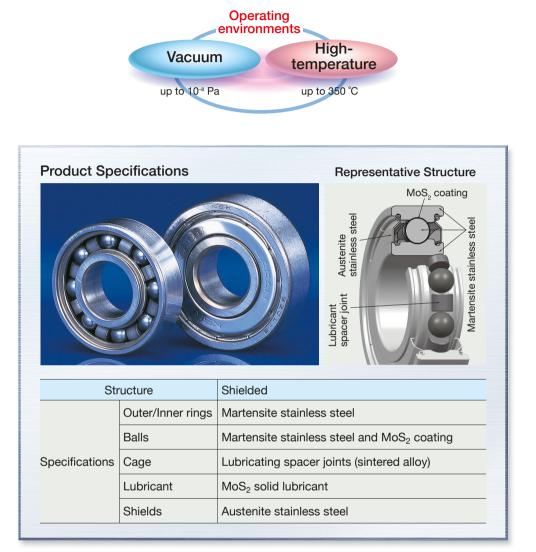
Applications: Ion implantation equipment, sputtering equipment, vacuum vapor deposition equipment
