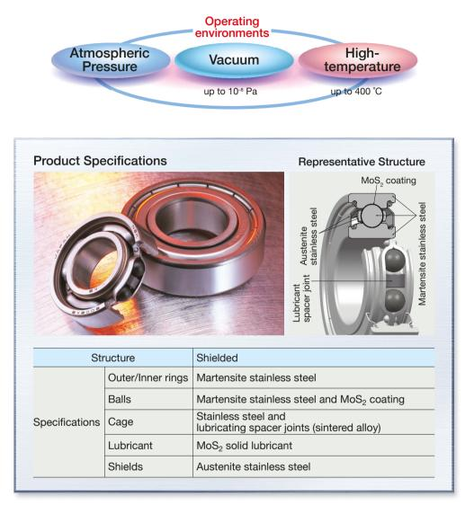
Applications: Vacuum vapor deposition equipment, kilns, kiln cars, steel plants, high-temperature conveyance equipment
