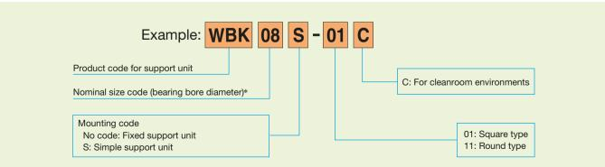
\* For simple support units, please note that size codes of 12 or less do not represent bearing bore diameters.
