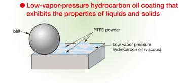
Flake-shaped PTFE powder increases the surface area for adhered lubricant, increasing lubricant retention.
