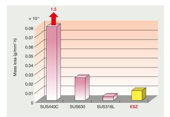
Results of sodium hypochlorite solution immersion test
