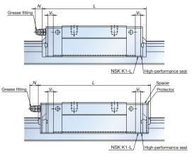
Dimensions of a linear guide equipped with high-performance seals and NSK K1-L
