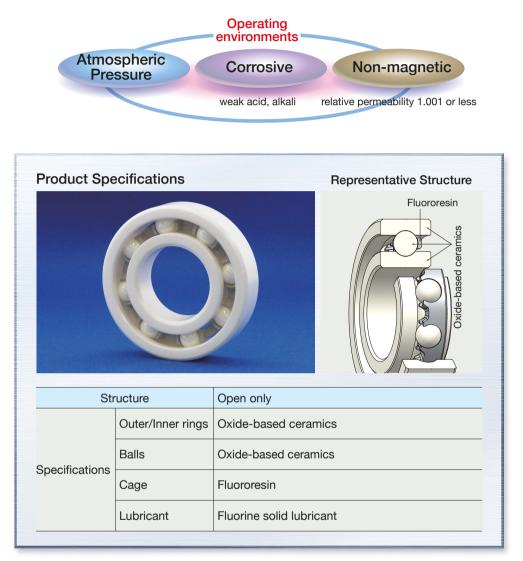
Applications: Corrosive environments: Semiconductor production machinery, chemical processing equipment, metal plating equipment Non-magnetic requirements: Electron beam drawing devices, electron beam exposure equipment, inspection equipment
