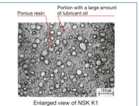
Made of porous synthetic resin containing a large amount of lubrication oil. When moved to contact the raceway surface, NSK K1 supplies fresh lubricating oil.
