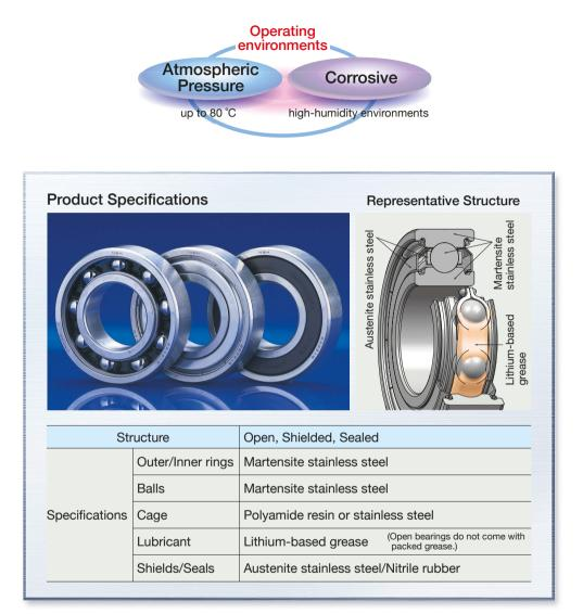
Applications: Equipment used in high-humidity environments: food processing, cleaning, chemical processing, fishery equipment
