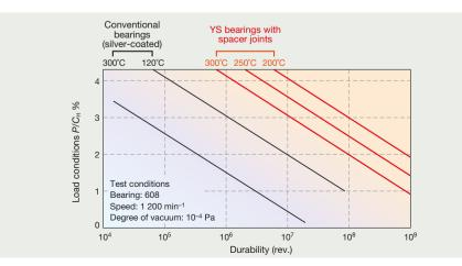
YS Bearings with Spacer Joints
