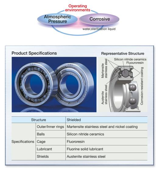
Applications: Semiconductor/FPD/HD cleaning equipment, etching equipment, food processing machinery, various conveyor lines
