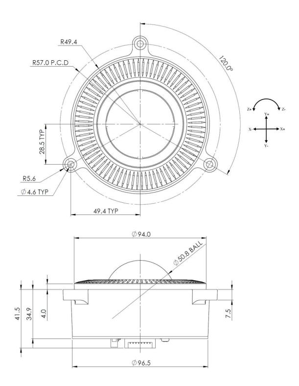
Dimensional drawing specifies factory default orientation. All dimensions are in mm unless otherwise stated. Tolerances +/-0.2mm unless otherwise stated
