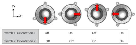
Figure.1 Mounting Orientations
