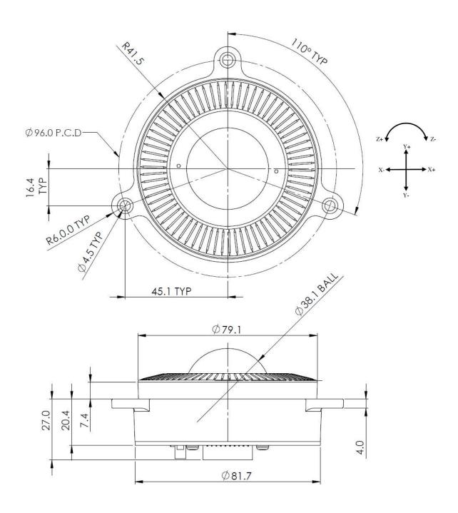
Dimensional drawing specifies factory default orientation. All dimensions are in mm unless otherwise stated. Tolerances +/- 0.2mm unless otherwise stated
