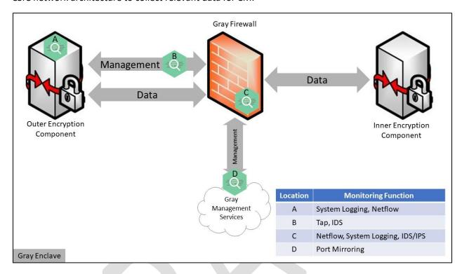
Figure 4. Examples of Monitoring Functions
