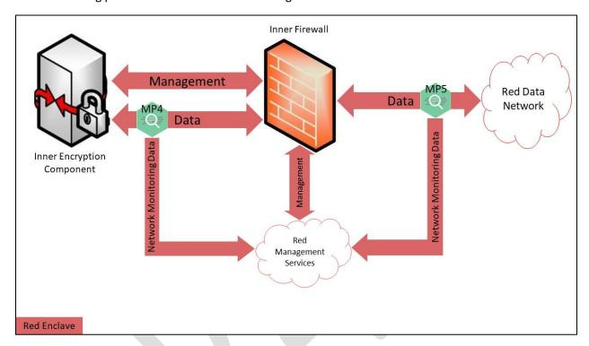
Figure 10. Monitoring Points 4 and 5: Red Data Line
