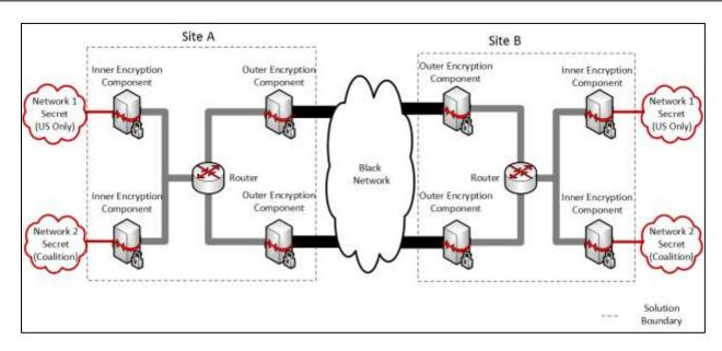
Figure 9. MSC Solution with Redundant Outer Encryption Components
