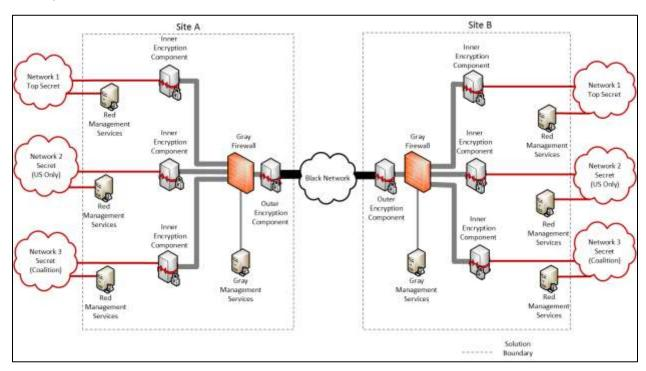
Figure 6. MSC Solution for Networks at Different Security Levels
