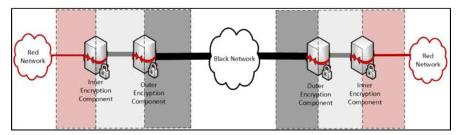
Figure 1. Two Encryption Tunnels Protect Data Across an Untrusted Network
