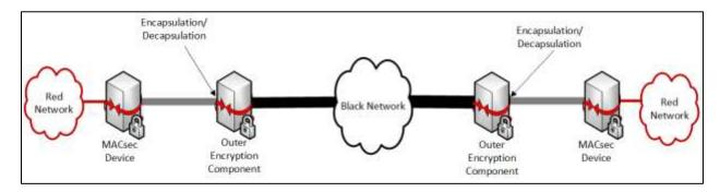
Figure 7. Encapsulating MACsec on an Internal Interface
