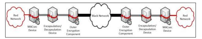
Figure 8. Encapsulating MACsec with a Separate Device
