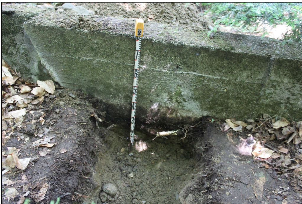
Photo 11. Dam #2, ASA 3, Test 2, placed against the south side of the concrete wall in the north end of the APE. Note dense sand and gravel beneath thin A horizon with concrete resting on gravel within the ditch. View to the north/northwest.
