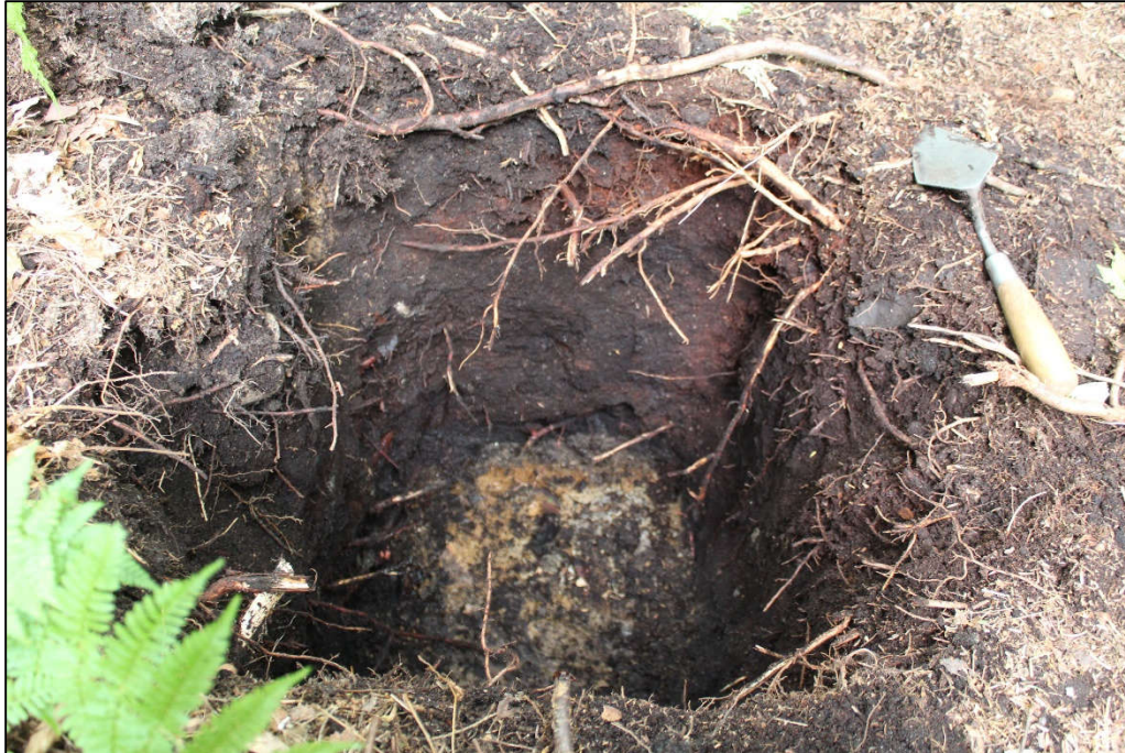
Photo 10. Dam #2, ASA 3, Test 7, north profile. Note thick A horizon over sand and gravel C horizon.
