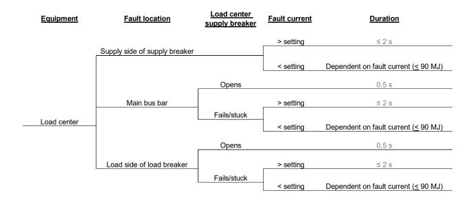
Figure 3-23 Zone 3 fault durations
