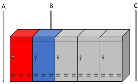
Figure G-4 Example 2: switchgear bank (normal supply in red; secondary supply in blue; conduits A, B, and C)
