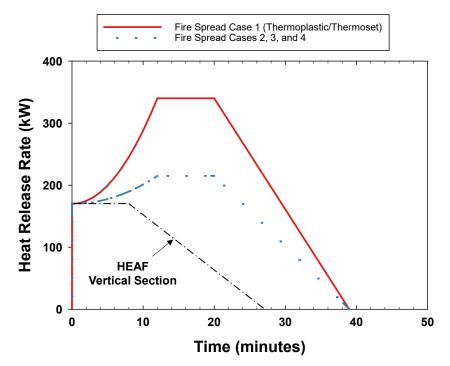
Figure 6-25 Total peak HRR profiles for a HEAF vertical section that ignites one adjacent vertical section
