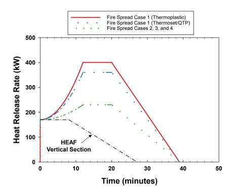
Figure 6-26 Total peak HRR profiles for a HEAF vertical section that ignites two adjacent vertical sections
