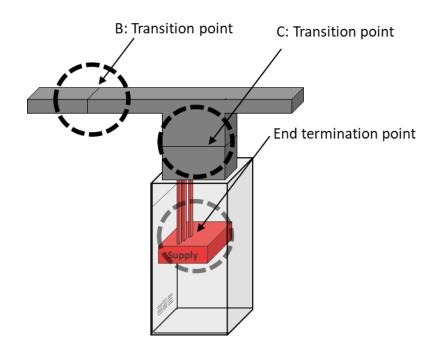
Figure 5-5 Transition point C from segmented bus duct with known transition points
