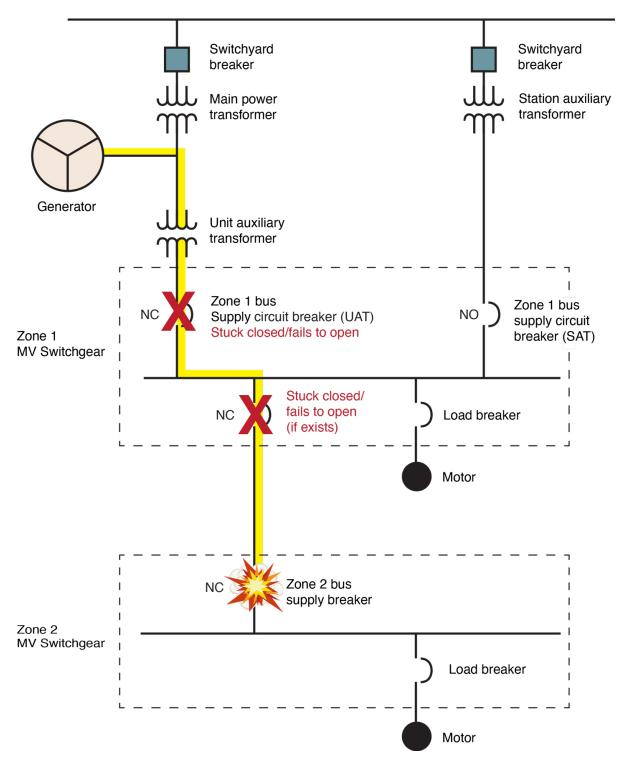
Figure 6-6 Example of a generator-fed fault (fault on Zone 2 with at least three independent failures)
