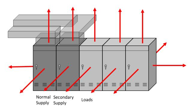
Figure 8-3 Application of MV switchgear screening ZOI
