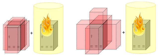
Figure 6-3 Energetic HEAF ZOI at short and long FCTs with ensuing fire (figures not to scale)
