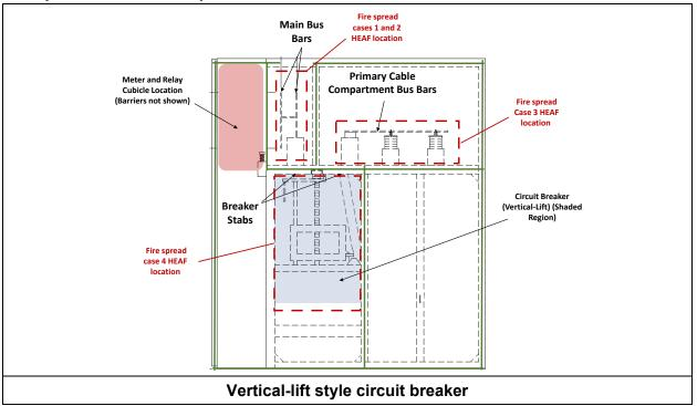
High Energy Arcing Fault Damage Criteria and Zone of Influence
