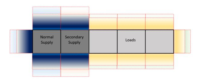
Figure 8-13 Overhead view of MV switchgear configuration-specific ZOIs: refinement level 2
