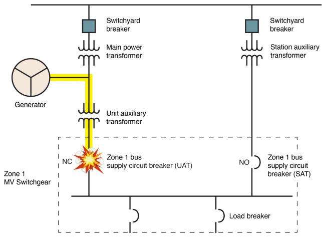
Figure 6-5 Conceptual drawing of a generator-fed fault with stuck Zone 1 bus supply circuit breaker
