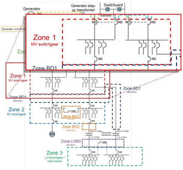
Figure 3-11 Zone 1: MV switchgear (Bin 16.b)
