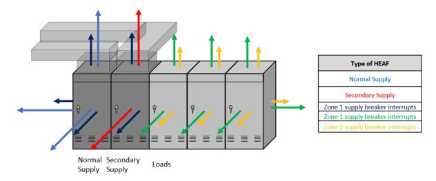
Figure 8-12 MV switchgear configuration-specific ZOIs: Refinement level 2
