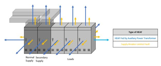
Figure G-5 Zone 2 MV switchgear refinement level 1 ZOIs
