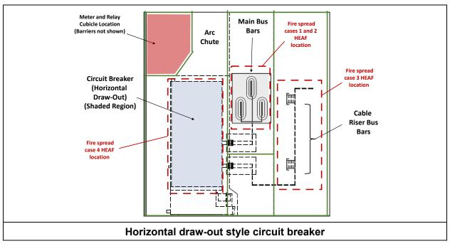
Figure 6-21 HEAF locations for each fire spread case
