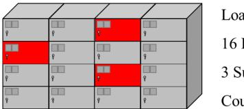
Load Center 16 Breakers in 4 Sections 3 Supply Breakers (red) Count = 3
