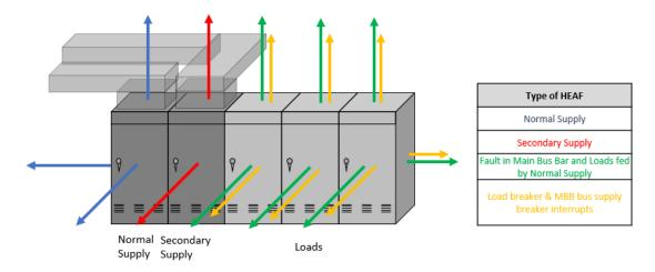
Figure 8-6 MV switchgear configuration-specific ZOIs
