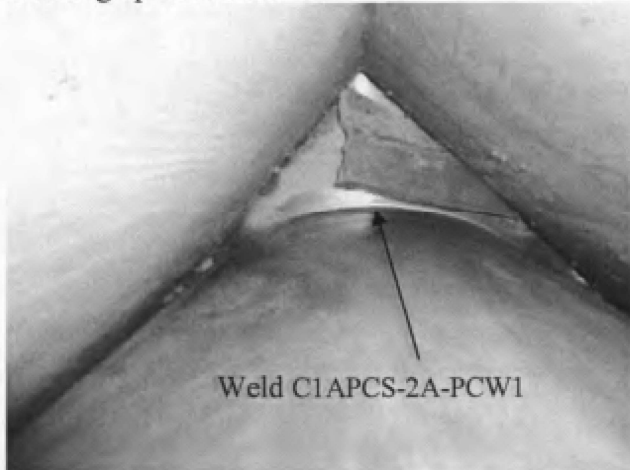
Figure 2.8-2 CIAPCS-2A-PCW1, Weld 24 Examination Location and Coverage Map
