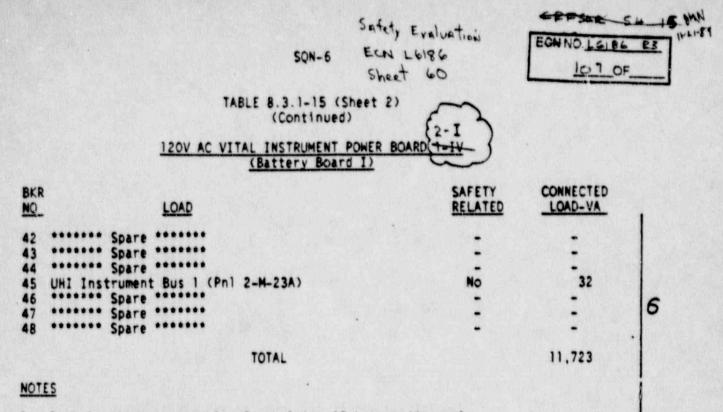
1. Each inverter is capable of supplying 15 kva continuously.
