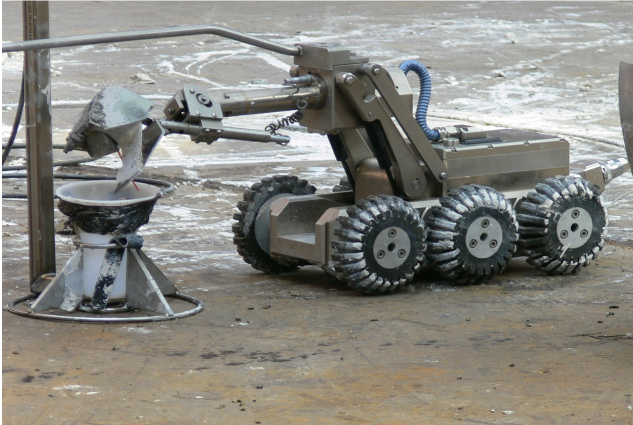
Figure 5-4. Off-Riser Sampling System Sampler.
