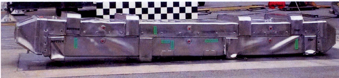
Figure 2-7 – Global Package Damage after Test CD3
