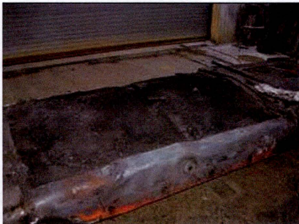
View of Lid After Outer Shell Removal
