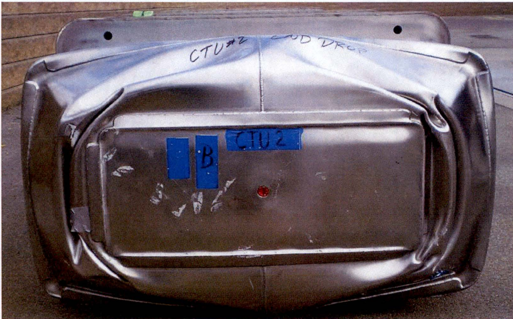
Figure 2-5 – Front View of Impact Limiter Damage
