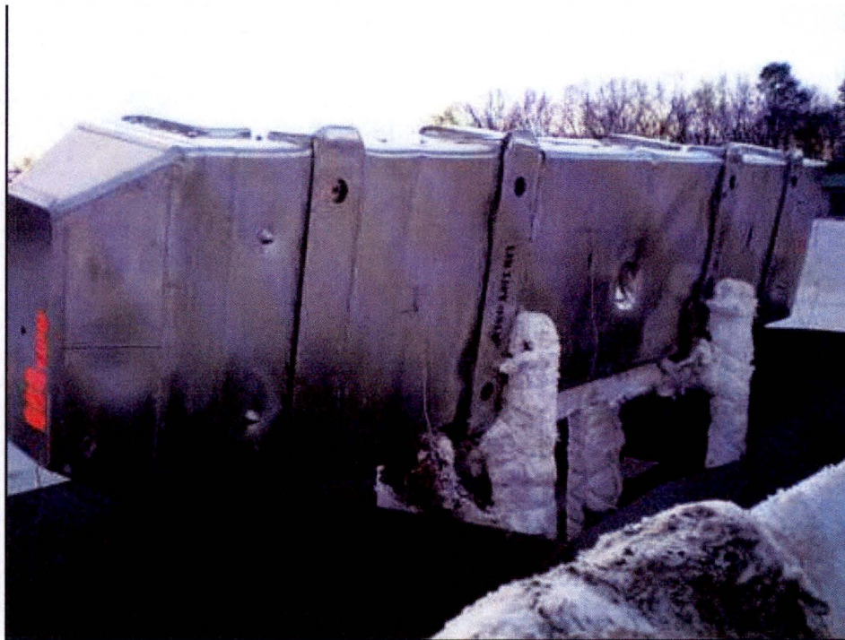
Figure 3-6 – MAP CTU 3 Mounted on Insulated Test Stand within Weir
