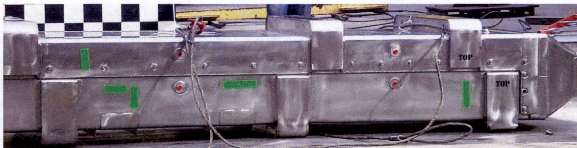
Figure 2-3 – Secondary Impact Stiffener Damage
