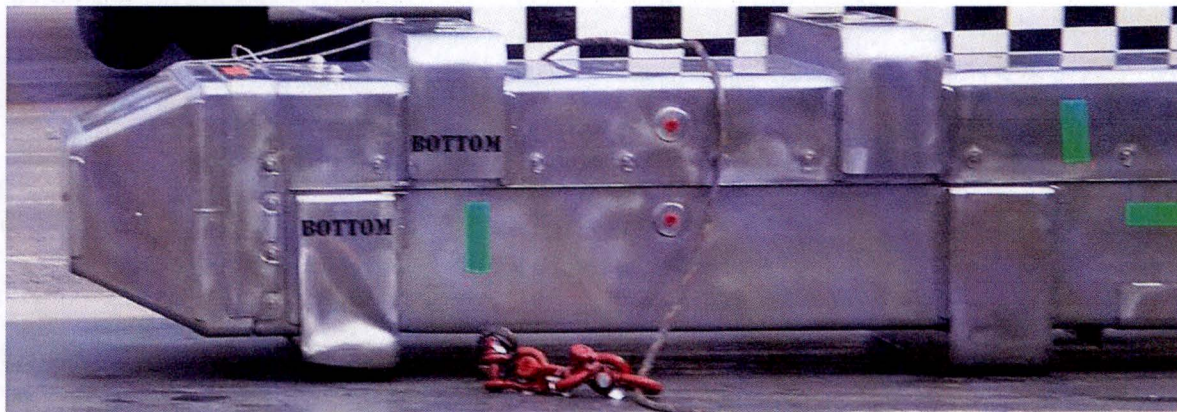
Figure 2-2 – Primary Impact Stiffener Damage
