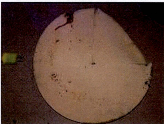
Figure 3-29 – Remaining 6 lb/ft 3 foam, backside
