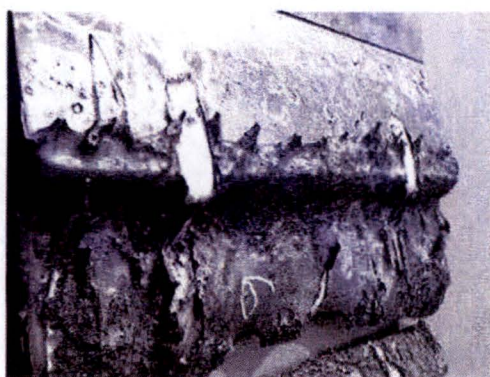
Figure 2.12.1-76 – Segment #5 melted piece
