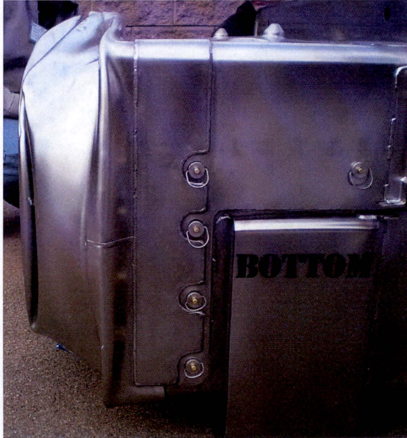
Figure 2-6 – Side View of Impact Limiter Damage
