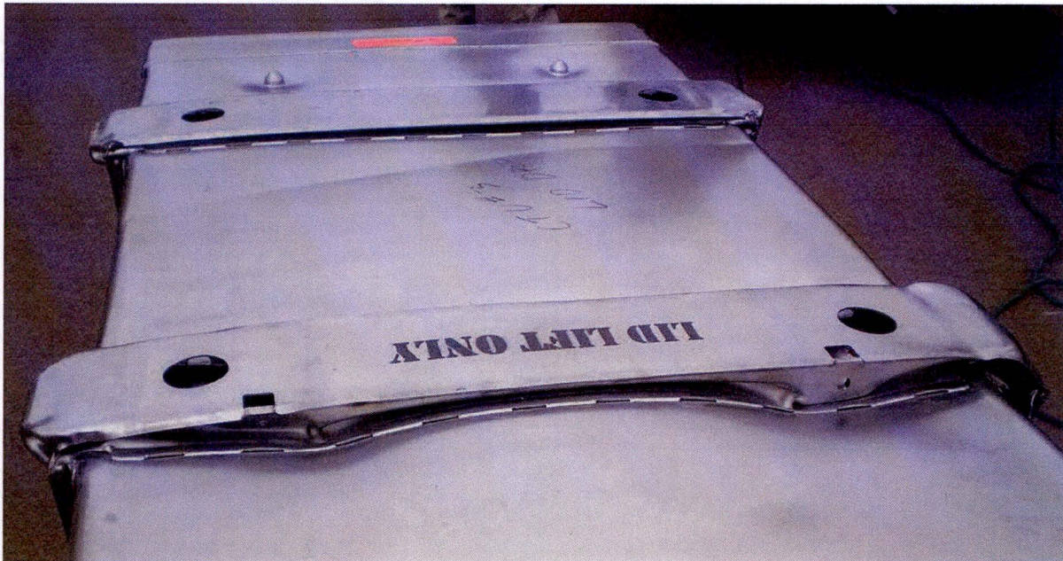
Figure 2-13 – Shell Deformation at Lid Lifting Locations
