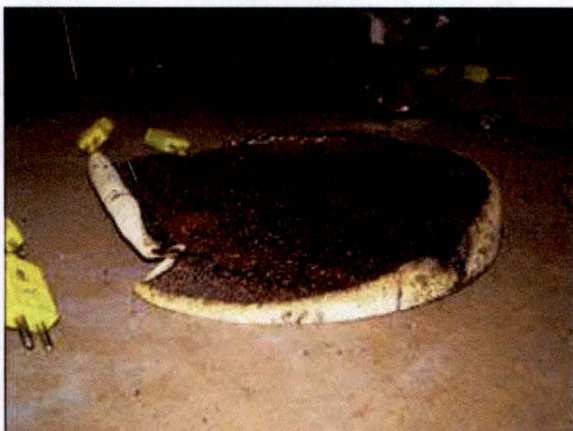
Figure 3-31 – Remaining 6 lb/ft 3 foam
