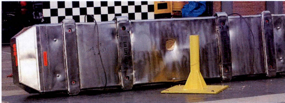
Figure 2-18 – Puncture Damage for Test CP3
