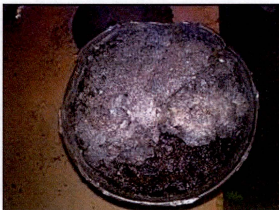
Figure 3-30 – Foam char under ceramic fiber paper
