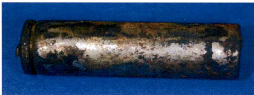
An 18650 cell that has undergone thermal runaway.
