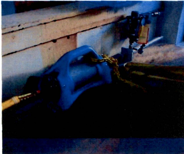
Figure 3.9 Tensile Test for Control Cable Housing
