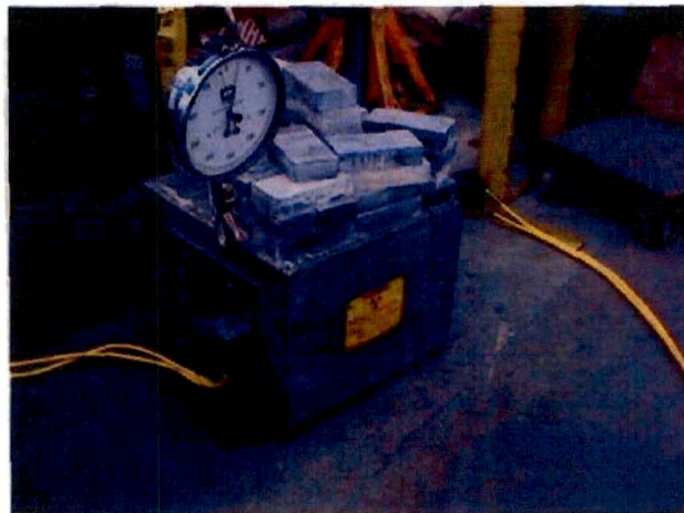
Figure 3.10 Tensile Test for Control Cable with Source Assembly
