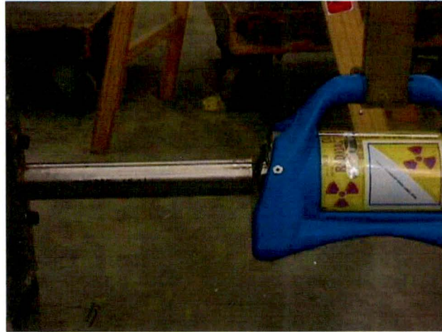
Figure 3.5 Horizontal Shock on Front Knob
