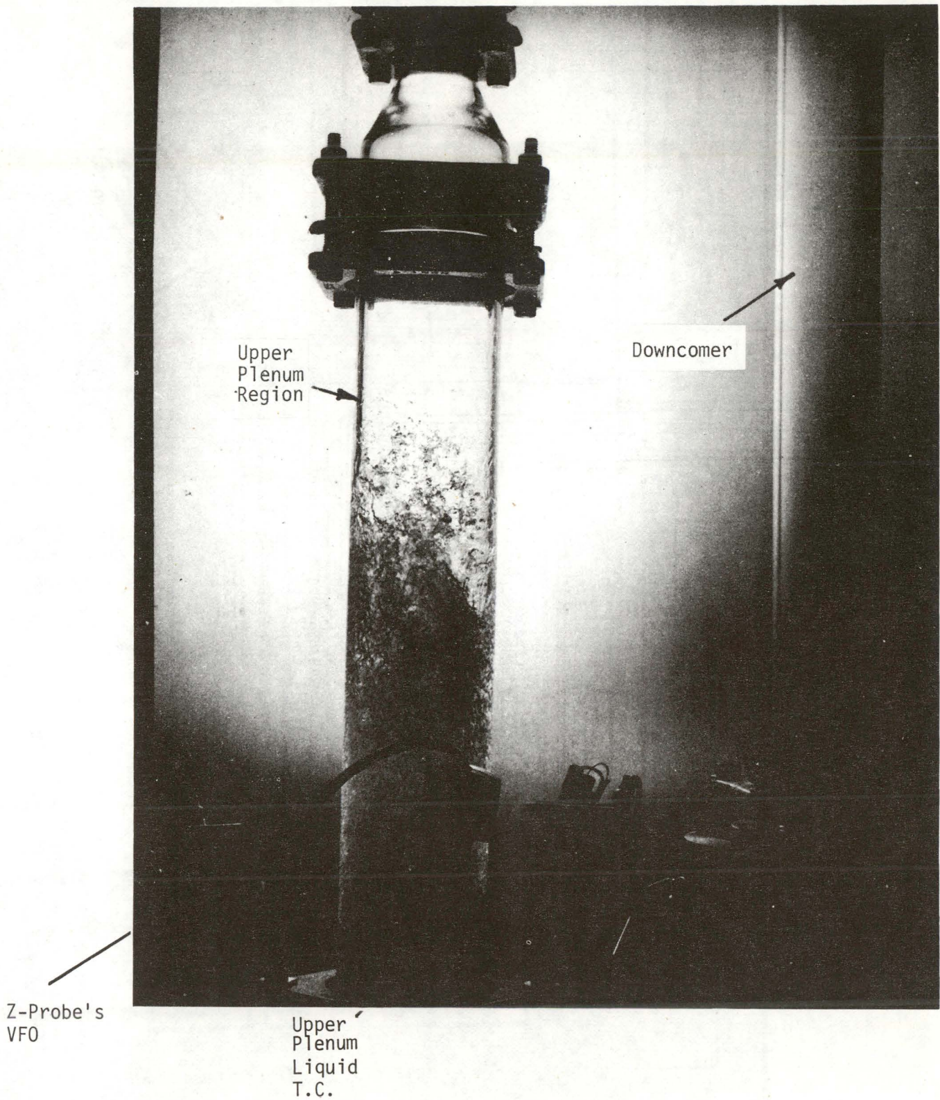
Figure-11f Two-Phase Mixture in Upper Plenum of PCE Test Section
