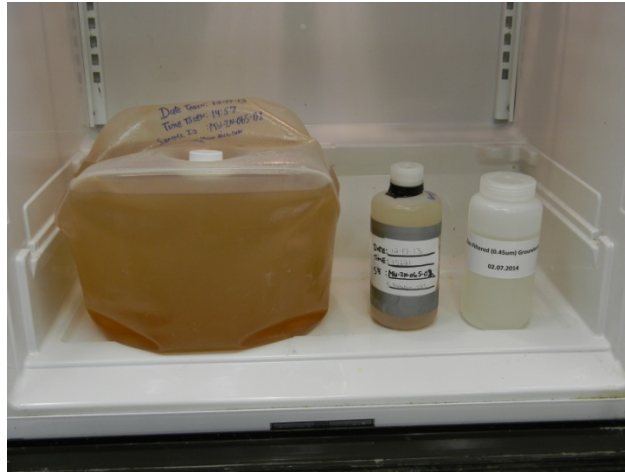
Figure 6. Groundwater solutions received from ZionSolutions (the one liter wide-mouth bottle with the clear solution on the right of the photograph is Zion groundwater that had been filtered using a 0.45 \mu\text{m} filter membrane)
