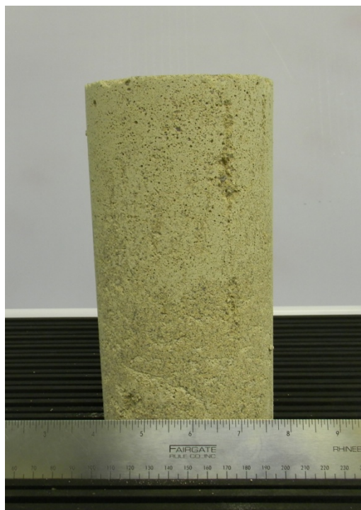
Figure 5. Low Density Cylindrical Grout form (CLS02 426-14) removed from the plastic container following 41 days of curing.
