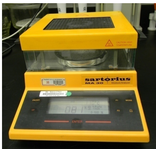
Figure 8. The Sartorius MA 30 Moisture Analyzer used to measure the moisture content of the three different materials used in this sorption study. (Note the photograph on the right (open lid) shows a Cinder Block sample visible in the aluminum dish.)
