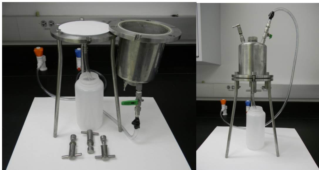
Figure 10. Filtering apparatus used to filter (filter membrane pore size is 0.45 \mu\text{m} ) the majority of groundwater received from ZionSolutions prior to the experiment start.
