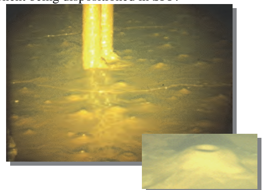
Sludge consists of insoluble solids that settle to the bottom of a tank. Note the offgas bubbles, including hydrogen generated from radiolysis.
