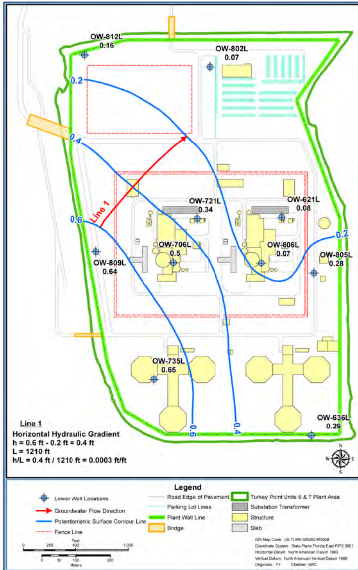
Figure 2.3-74 Biscayne Aquifer Potentiometric Surface Map, Lower Monitoring Interval, June 15, 2010 (Sheet 2 of 2) Low Tide
