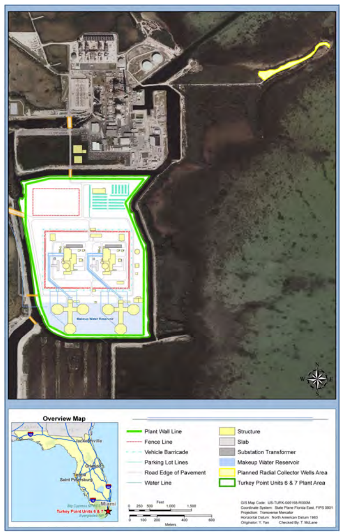
Figure 2.3-64 Radial Collector Well Area
