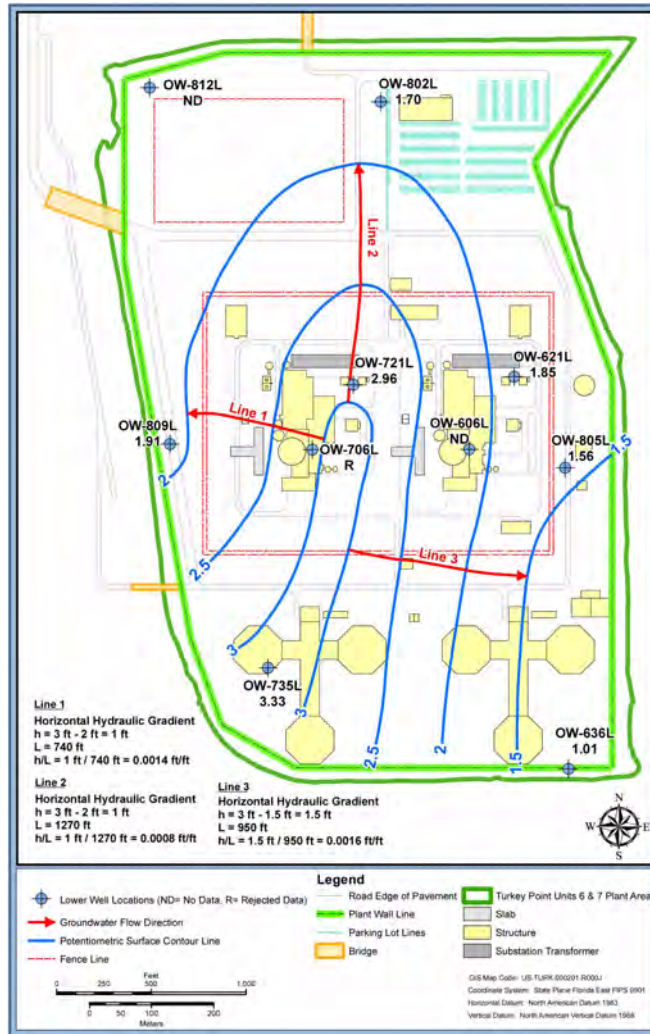
Figure 2.3-33 Biscayne Aquifer Potentiometric Surface Map, Lower Monitoring Interval, October 5, 2008 (Sheet 2 of 2) Low Tide
