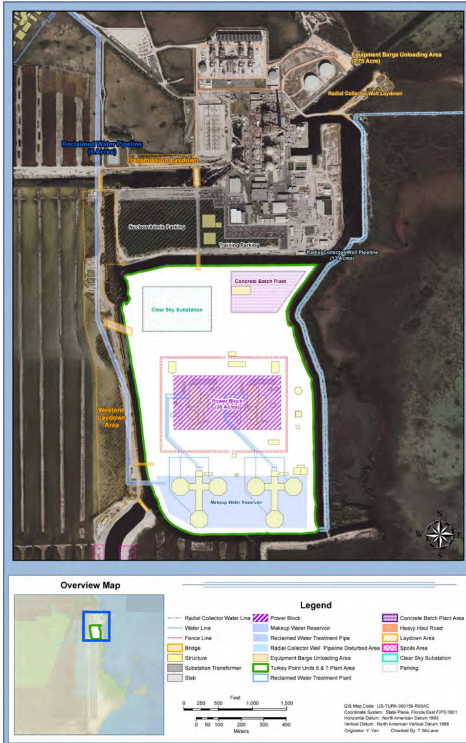
Figure 3.9-1 Construction Utilization Plan (Sheet 1 of 4)
