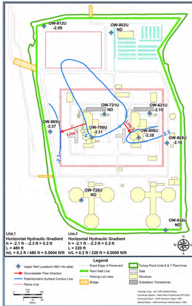
Figure 2.3-34 Biscayne Aquifer Potentiometric Surface Map, Upper Monitoring Interval, January 20-21, 2009 (Sheet 1 of 2) High Tide
