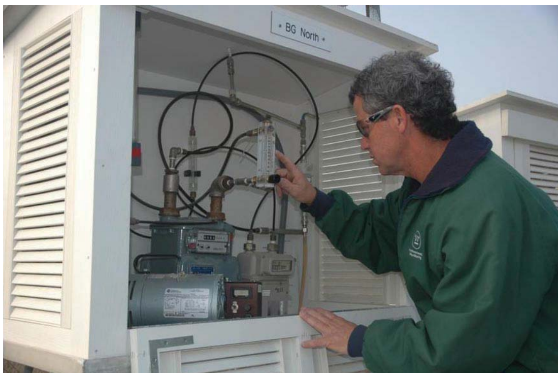
Figure 5-2 Environmental Monitoring Field Technician Reads Air Flow at the Burial Ground North Air Surveillance Station
