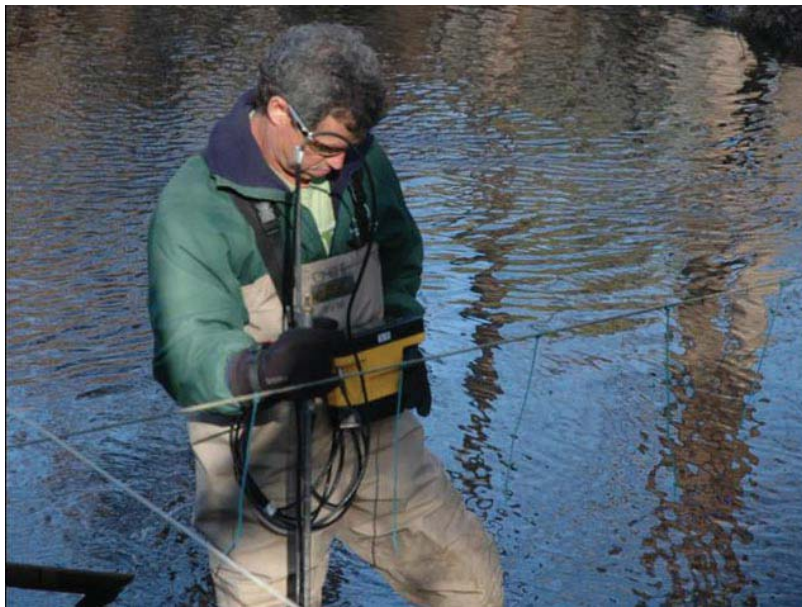
Figure 5-10 Environmental Monitoring Field Technician Performs Area Velocity Measurements across a SRS Stream
