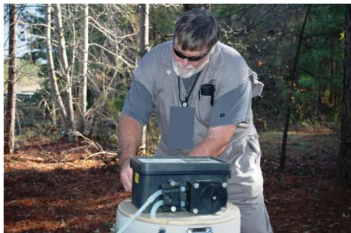
Figure 4-7 An Automated Water Sampler Programmed at an Industrial Wastewater Outfall
