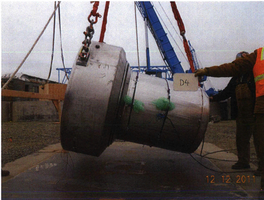
Figure 2.12.3-40 – Free Drop Test D4N/D4H Orientation
