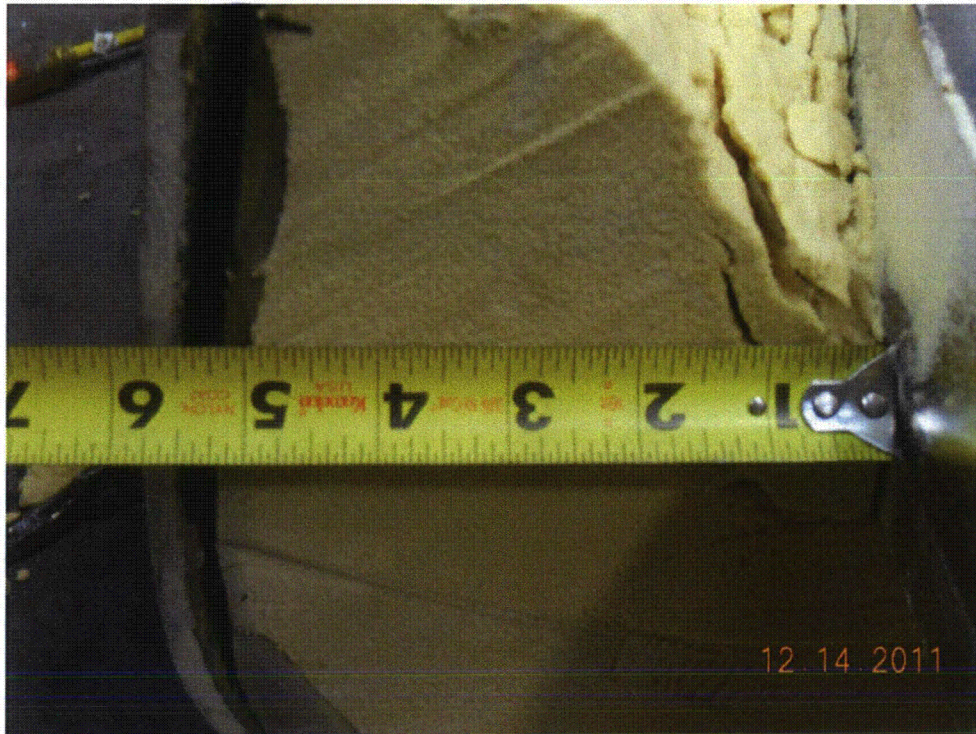
Figure 2.12.3-48 – Minimum Foam Remaining After Free Drop D4H
