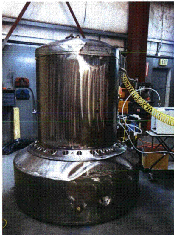
Figure 2.12.3-41 – CTU #2 Condition After Free Drop Test D4H (Also Showing P4)
