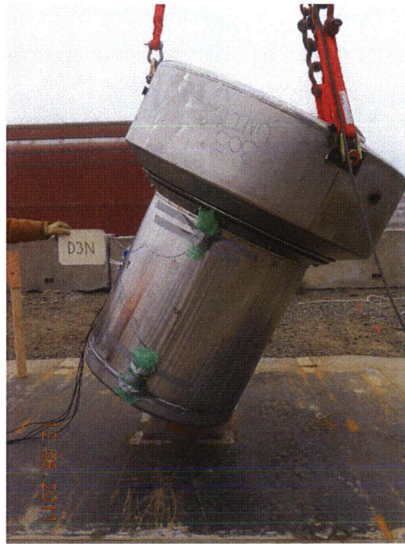
Figure 2.12.3-22 – Free Drop Test D3N/D3H Orientation
