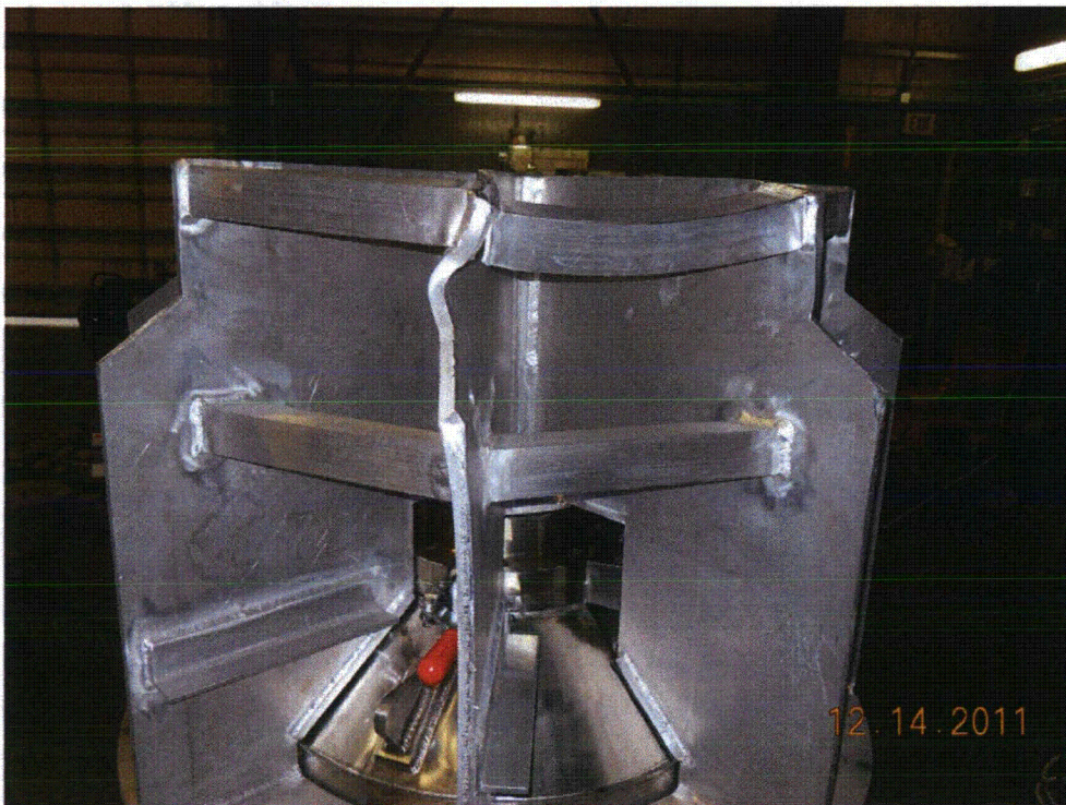
Figure 2.12.3-47 – Damage to Lodgment After Test Series D3 and D4
