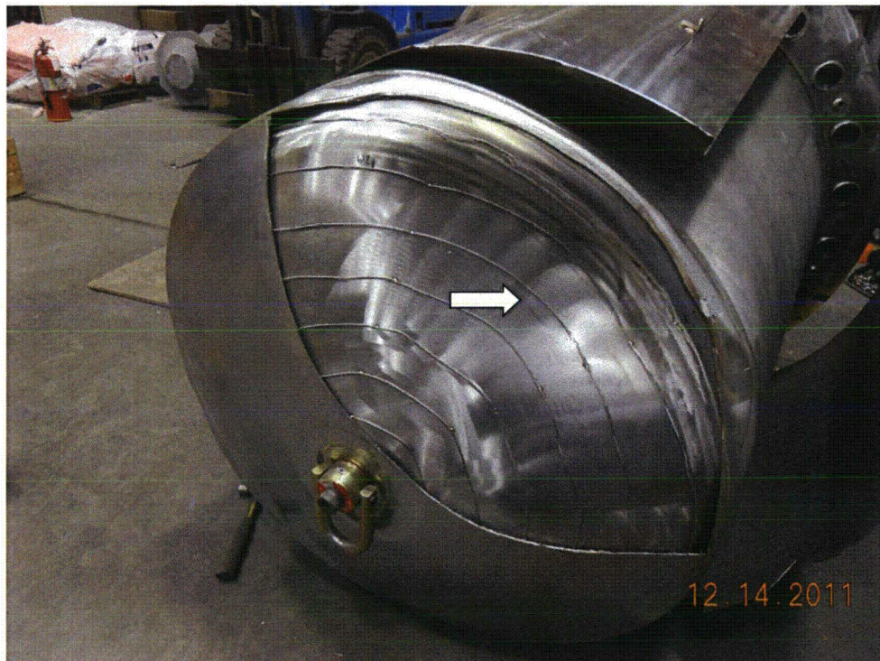
Figure 2.12.3-45 – View of Damage Due to Test Series D3, Head Shield Cut Away (arrow indicates puncture bar impact location)
