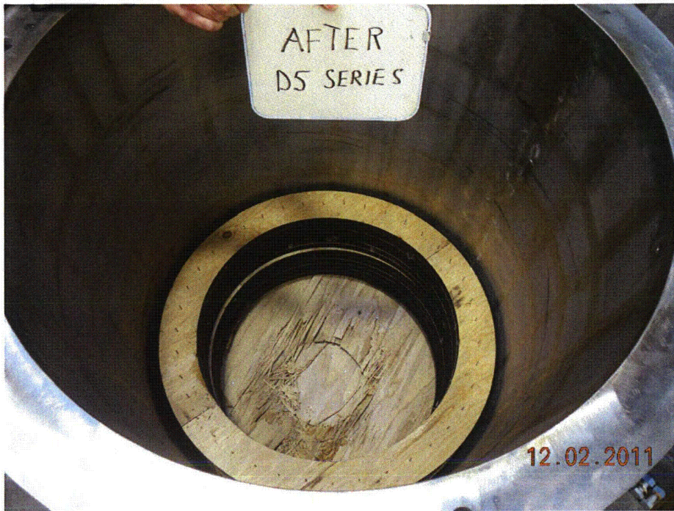
Figure 2.12.3-14 – Inner Container Lower Dunnage After D5 Test Series
