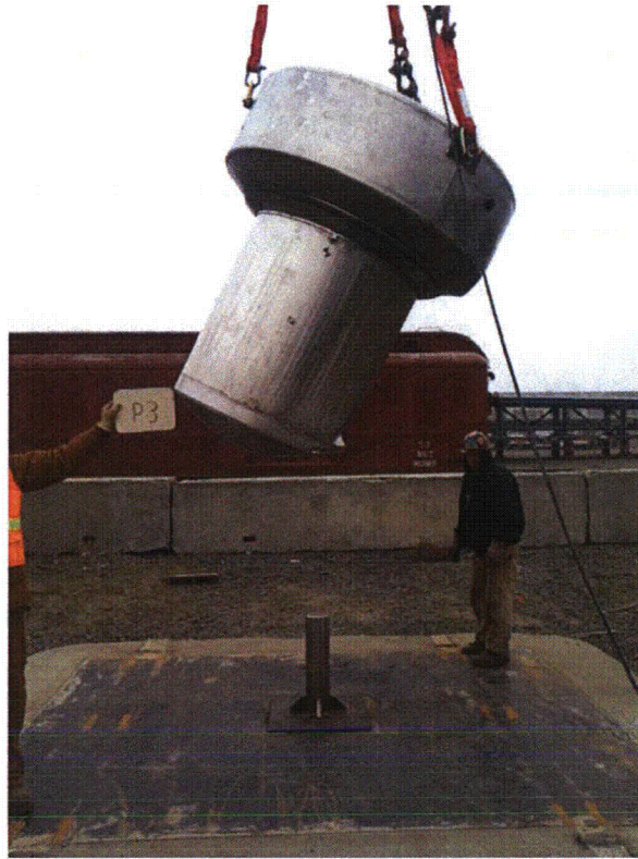
Figure 2.12.3-24 – Puncture Drop Test P3 Orientation
