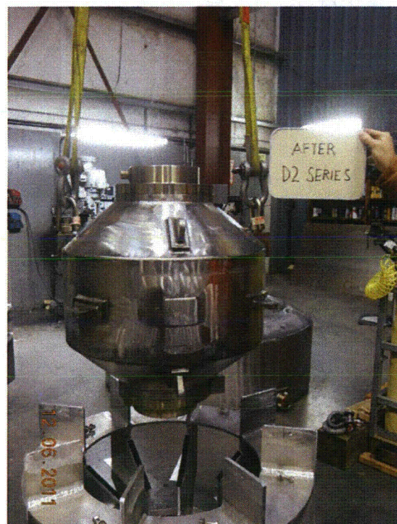
Figure 2.12.3-21 – Condition of LTSS After D1 and D2 Test Series
