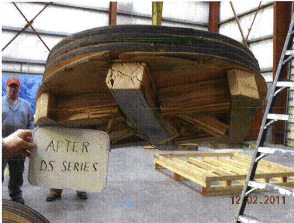
Figure 2.12.3-15 – Detail of Lower Dunnage Damage After D5 Test Series
