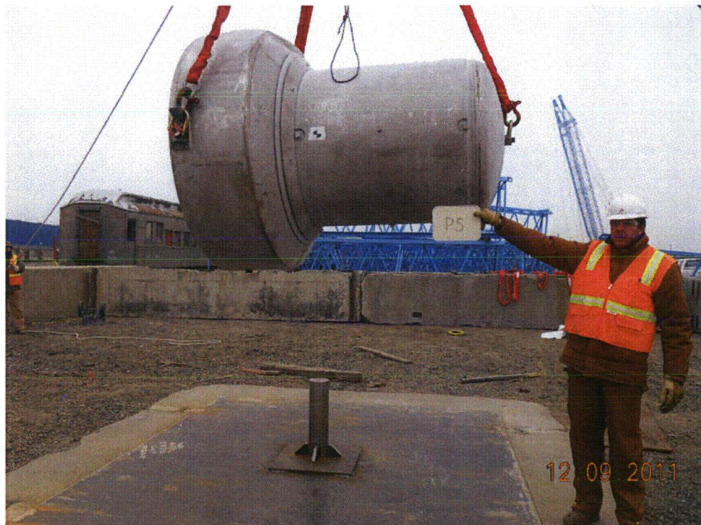
Figure 2.12.3-31 – Puncture Drop Test P5 Orientation
