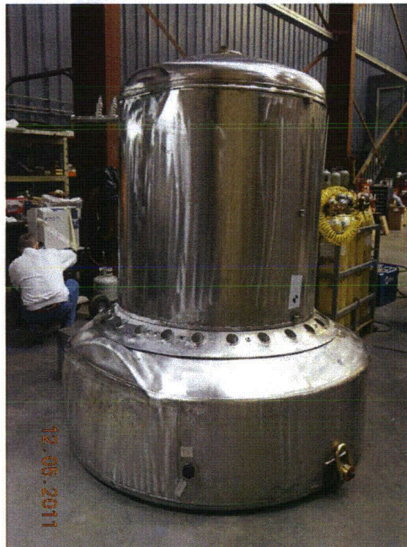
Figure 2.12.3-17 – CTU #1 Condition After Free Drop Test D2H
