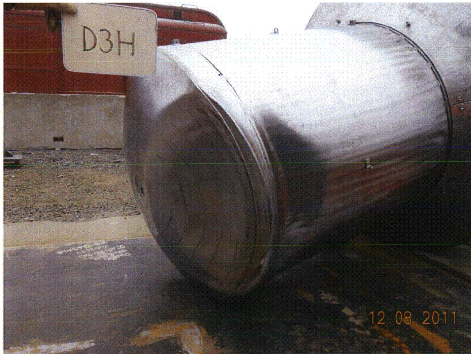
Figure 2.12.3-23 – CTU #2 Condition After Free Drop Test D3H
