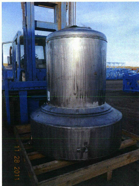
Figure 2.12.3-5 – CTU #1 Condition After Free Drop Test D1H
