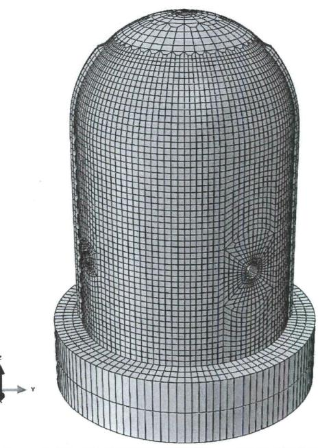
Figure 3: Model 3 – Meshed Shell Elements with Thickness Rendered (Still Under Development)
