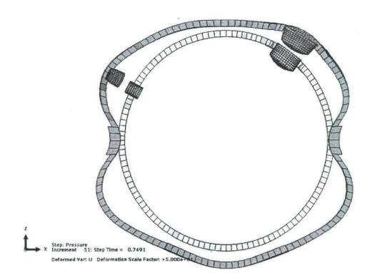
Figure 4: Deformed Shape at 3.0 x Design Pressure (x50) Highlighting Excessive Stiffness at Buttresses
