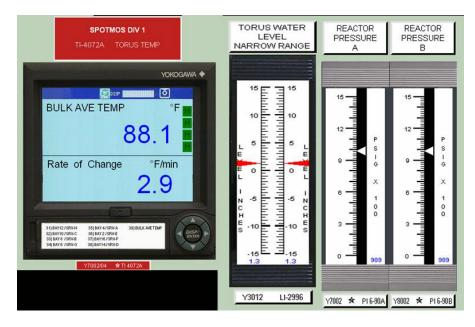
Of the times below, when will the Torus Heat Capacity Limit (Detail M) <u>**FIRST**</u> be exceeded? (Assume Torus temperature rate of change, Torus water level and Reactor pressure remain constant. Detail M is on the following page).
