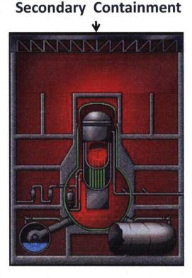
No Primary Containment Cooling therefore Primary Containment Overpressure-Vent to Secondary Containment
