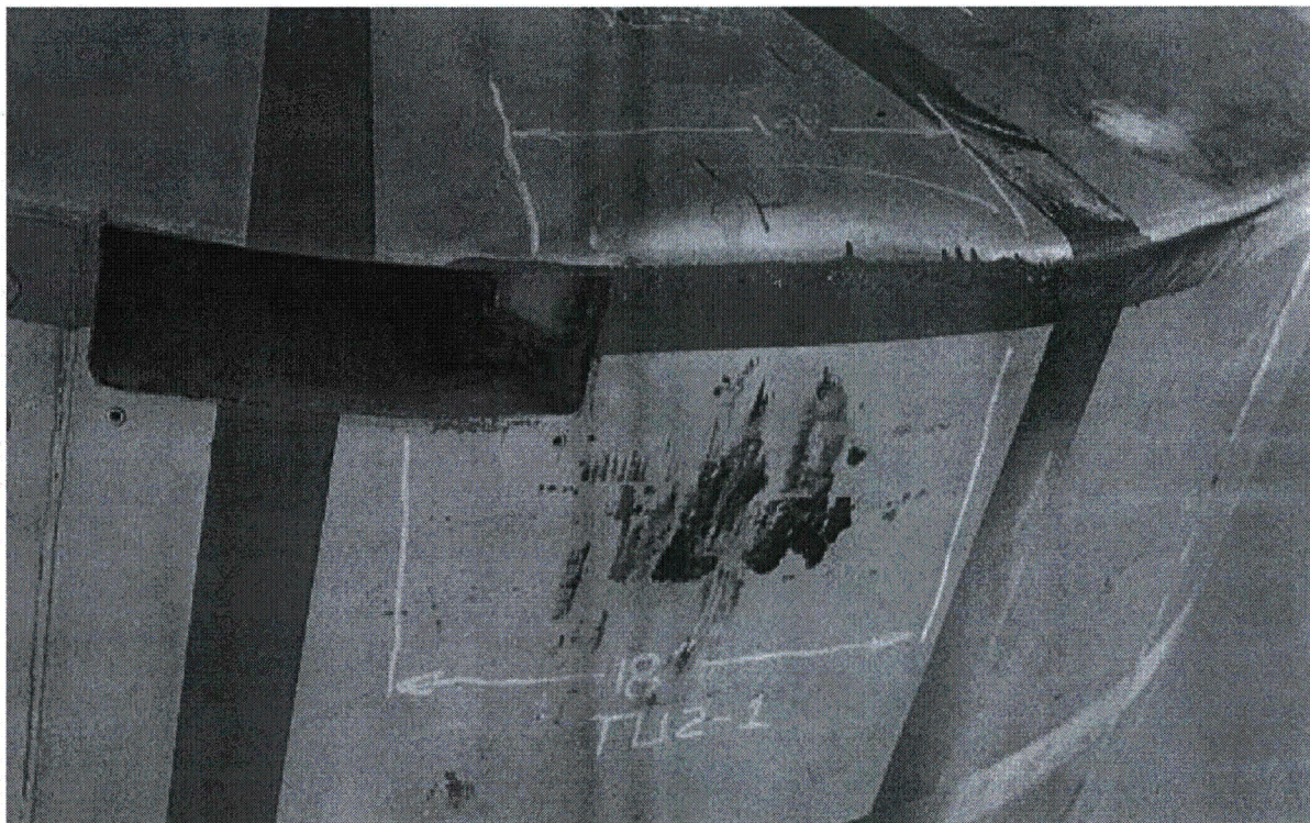
Figure 2.10.3-29 – CTU-1 Free Drop No. 1; Post-Drop Damage at Bottom (Body)
