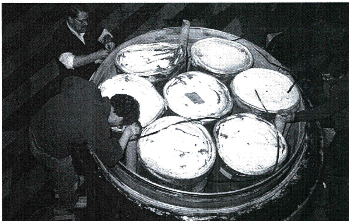
Figure 2.10.3-52 – CTU-1 Disassembly; Payload Drum Removal
