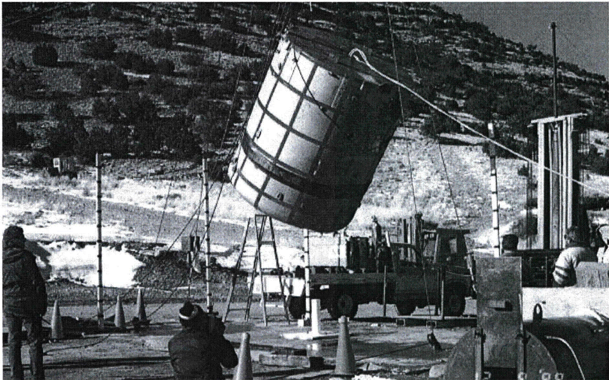
Figure 2.10.3-42 – CTU-1 Puncture Drop No. 8; Pre-Drop Positioning
