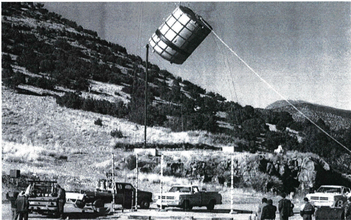
Figure 2.10.3-32 – CTU-1 Free Drop No. 3; Pre-Drop Positioning
