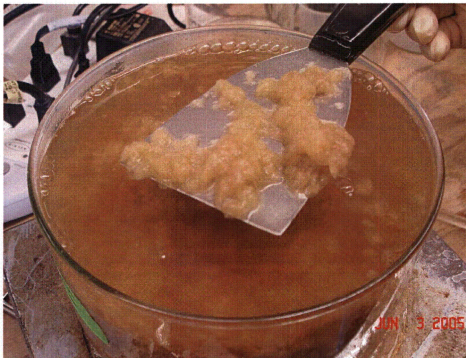
Figure 3-2. BP NUKON™. Figure 3. Blender Processed NUKON
