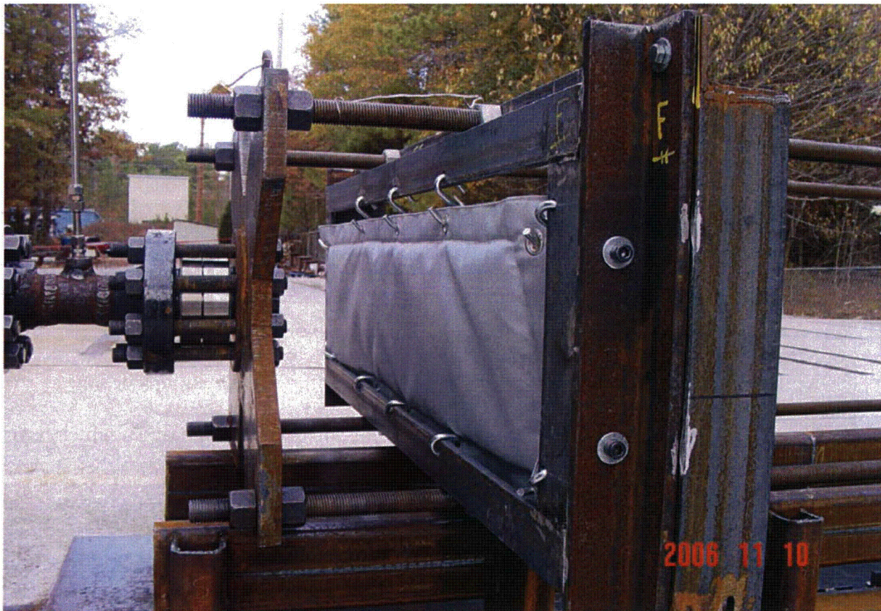
Figure 1: Lead Blanket #4 mounted prior to Jet Impingement Test Lead blanket specimen #4 secured at the top and bottom by hooks in the regularly spaced grommets to an open frame (open back).
