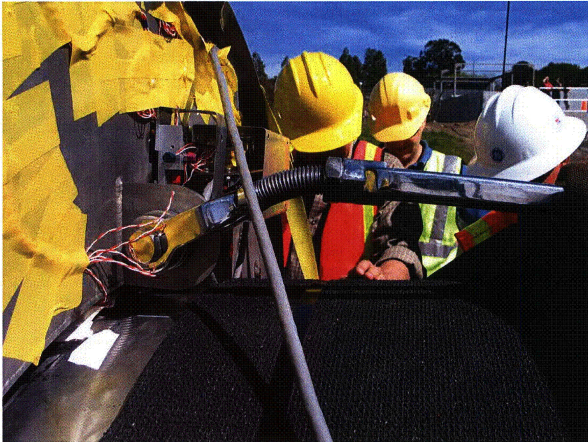
Figure 50 Uppermost turnbuckle after the slap-down drop.
