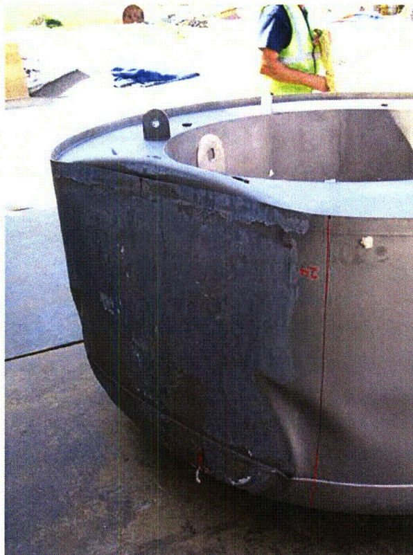
Figure 53 Damage to the impact limiter from the "slap-down" end of the cask.
