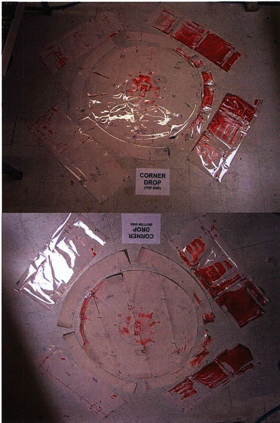
Figure 52 Pressure sensing film removed from the cask and impact limiters after the slap-down drop.
