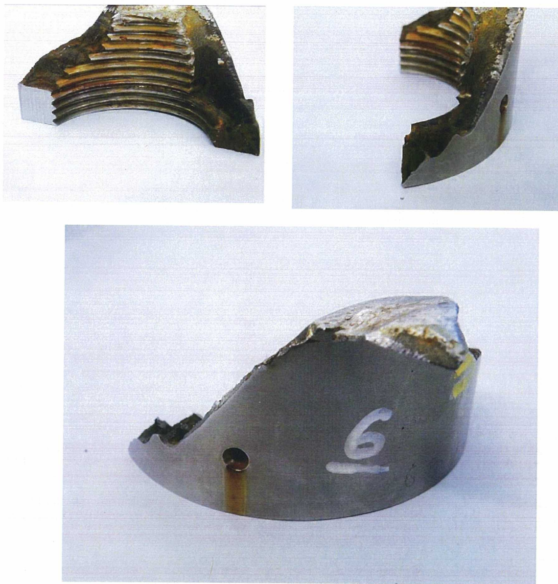
Figure 3-6: 11-P7C-6F showing Corrosion Deposit
