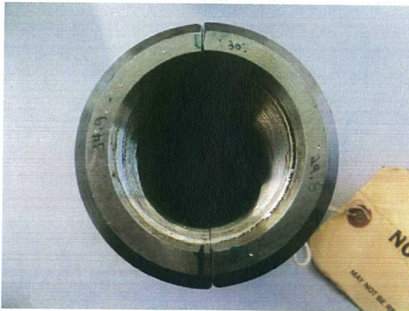
Hardness measurement indentations are present on both ends. Measurement values were 34.9, 30.7, 29.5 and 29.4 on motor end and 33.5, 32.2, 32.0 and 32.5 on impeller end.
