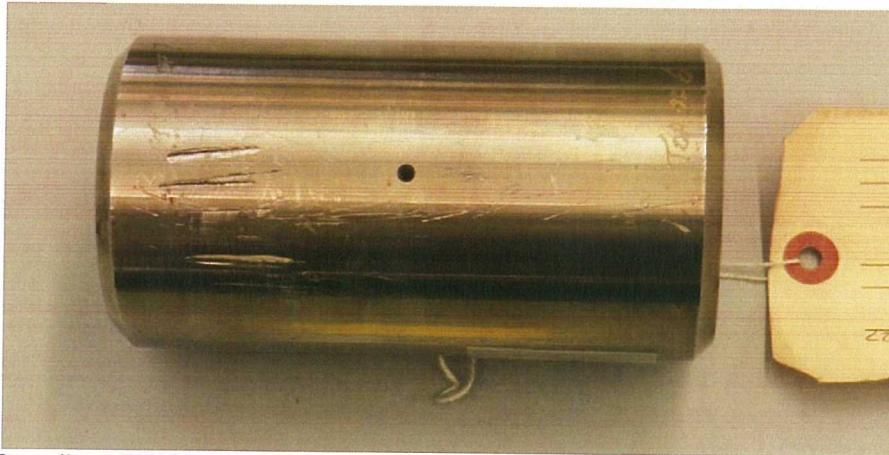
Coupling 11-PC-7 in as-received form. Shaft numbers engraved on the ends. Coupling exhibited wrenching marks on outer diameter.
