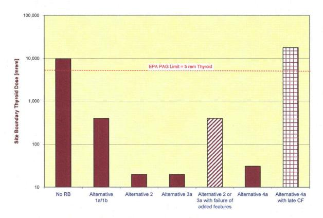
Figure 2. Comparison of PBMR NGNP Reactor Building Alternatives
