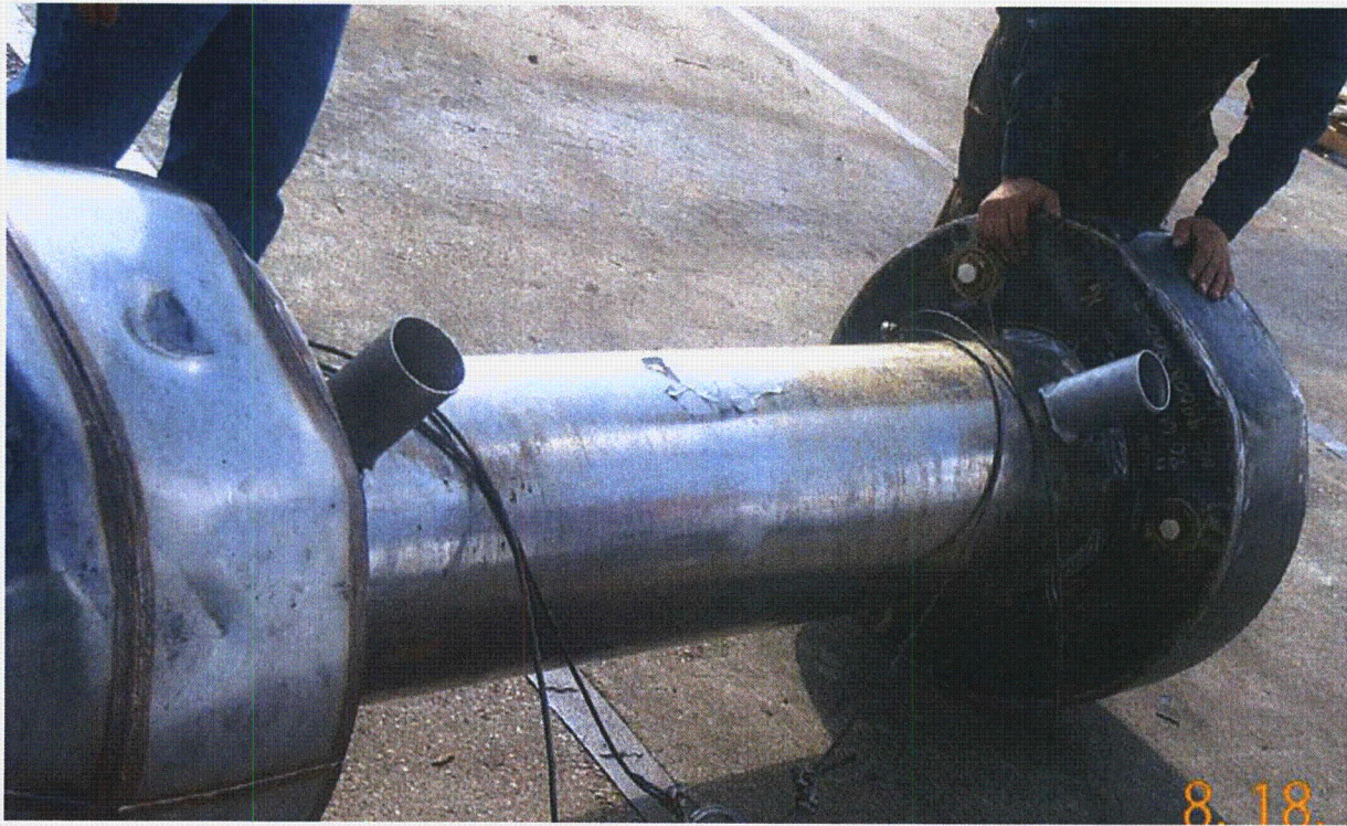
Figure 2.12.4-14 – ETU Test 6: View of Free Drop Damage
