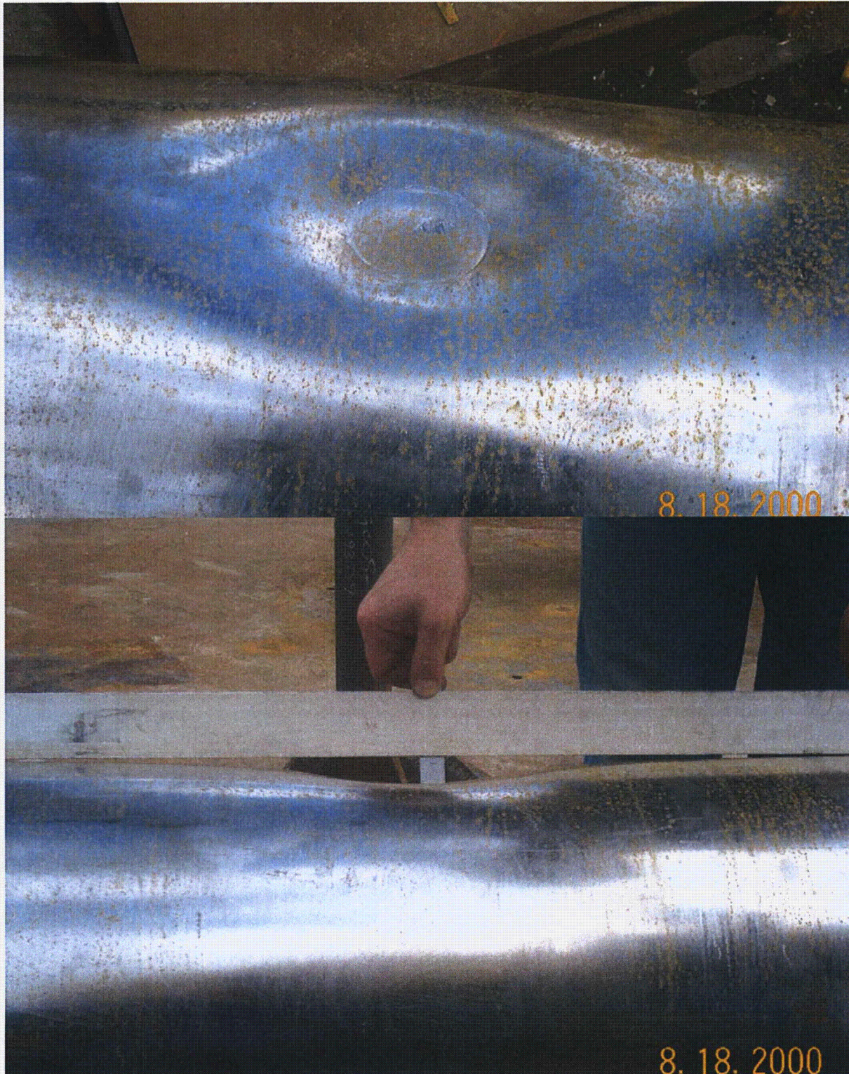
Figure 2.12.4-16 – ETU Test 7: View of Puncture Damage; ~1 \frac{1}{8} " Deep
