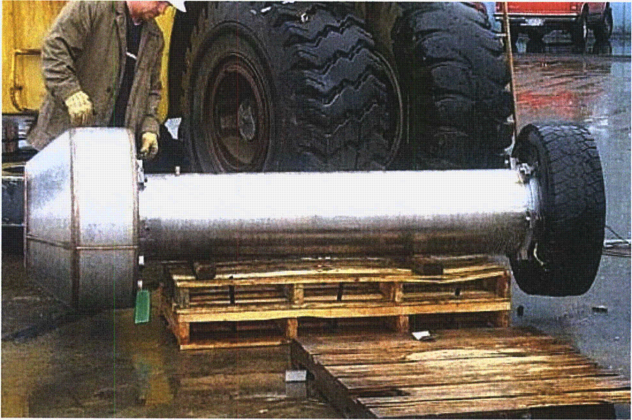
Figure 2.12.4-2 – ETU Initial Configuration (with Interim Impact Limiter)
