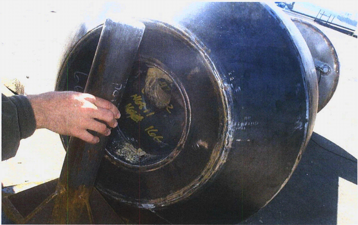
Figure 2.12.4-12 – ETU Test 5: View of Puncture Damage; ~2¾" Deep
