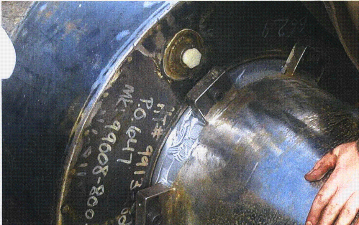
Figure 2.12.4-10 – ETU Test 4: View of Puncture Damage; ~3/8" Deep
