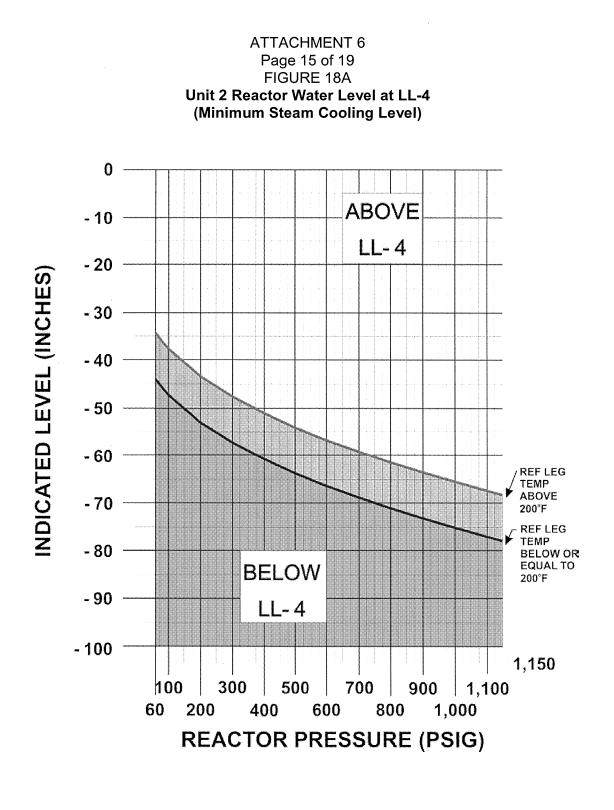
WHEN REACTOR PRESSURE IS LESS THAN 60 PSIG, USE INDICATED LEVEL. LL-4 IS -32.5 INCHES.
