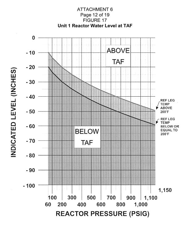
WHEN REACTOR PRESSURE IS LESS THAN 60 PSIG, USE INDICATED LEVEL. TAF IS -7.5 INCHES.
