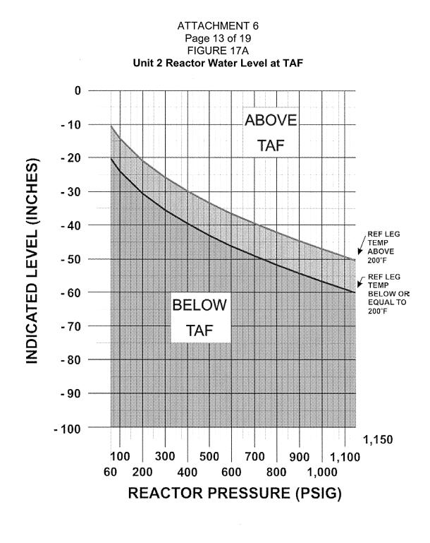
WHEN REACTOR PRESSURE IS LESS THAN 60 PSIG, USE INDICATED LEVEL. TAF IS -7.5 INCHES.
