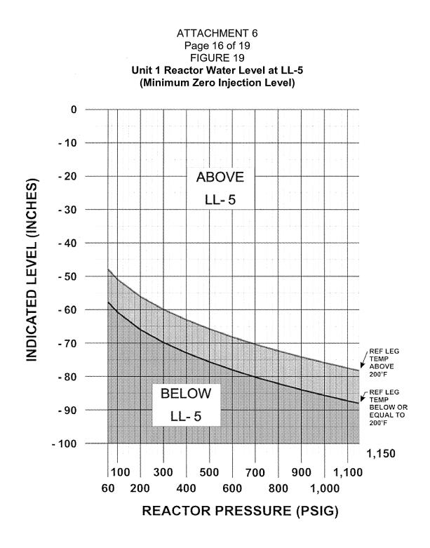
WHEN REACTOR PRESSURE IS LESS THAN 60 PSIG, USE INDICATED LEVEL. LL-5 IS -47.5 INCHES.
