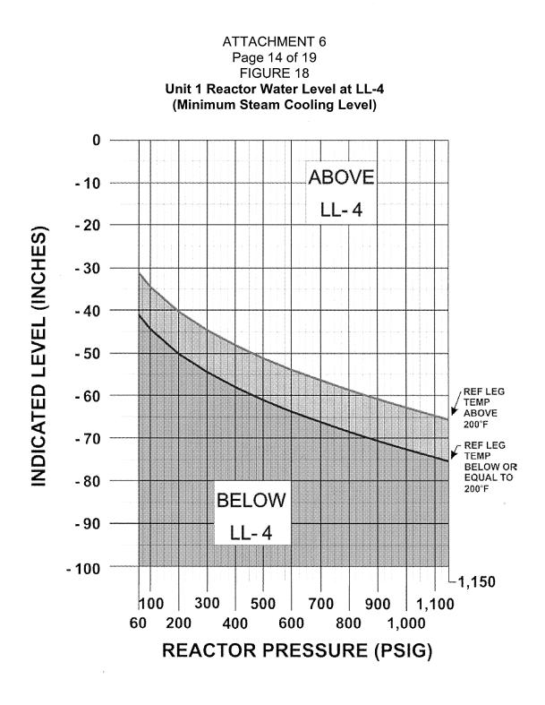
WHEN REACTOR PRESSURE IS LESS THAN 60 PSIG, USE INDICATED LEVEL. LL-4 IS -30.0 INCHES.
