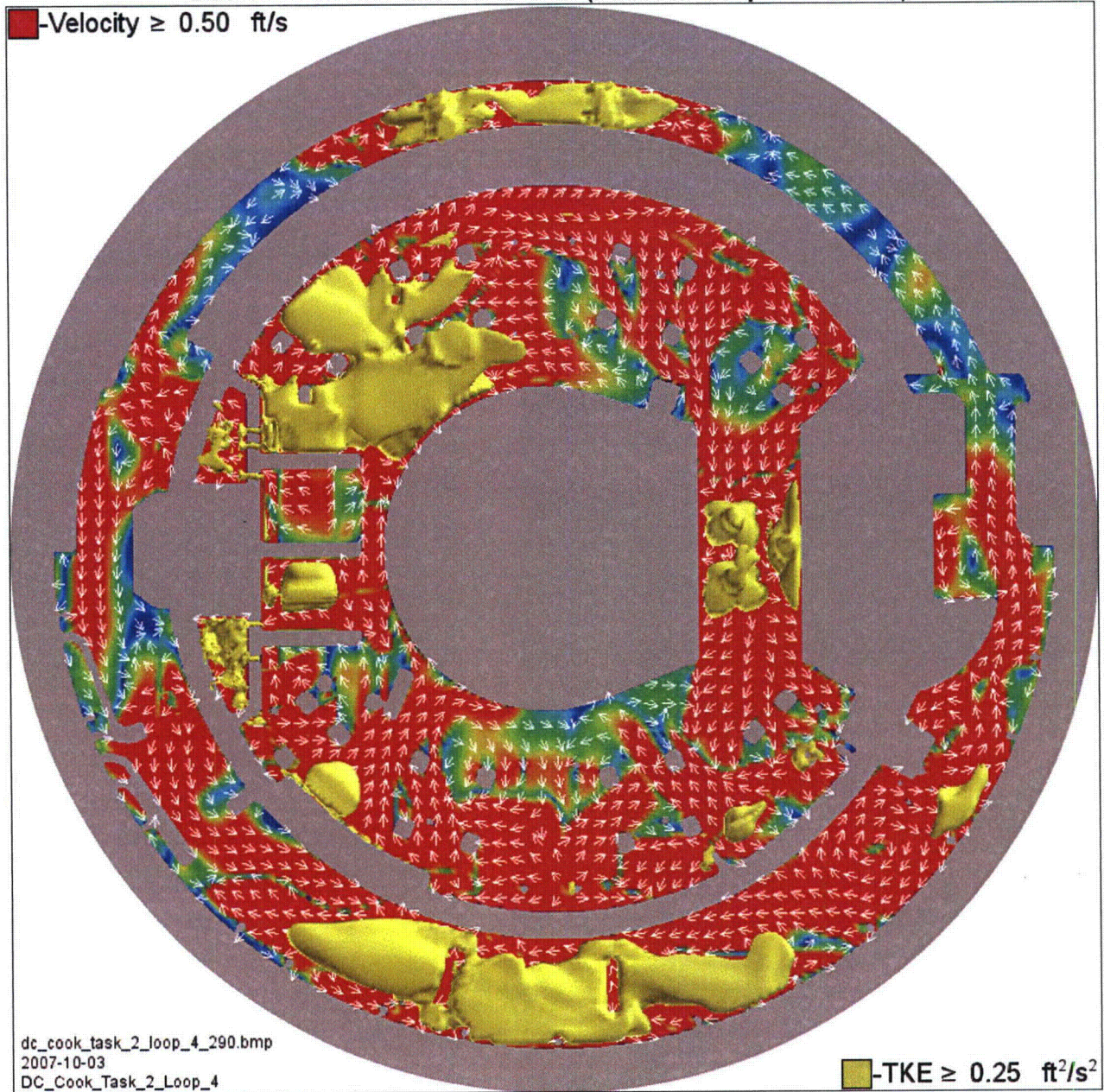
Figure 3e1-20 TKE and Velocity in the Pool at 290 Seconds - Just Before Restarting to Decrease the Ice Melt Flow Rate (Pool Fill Loop 4 CFD Run)
