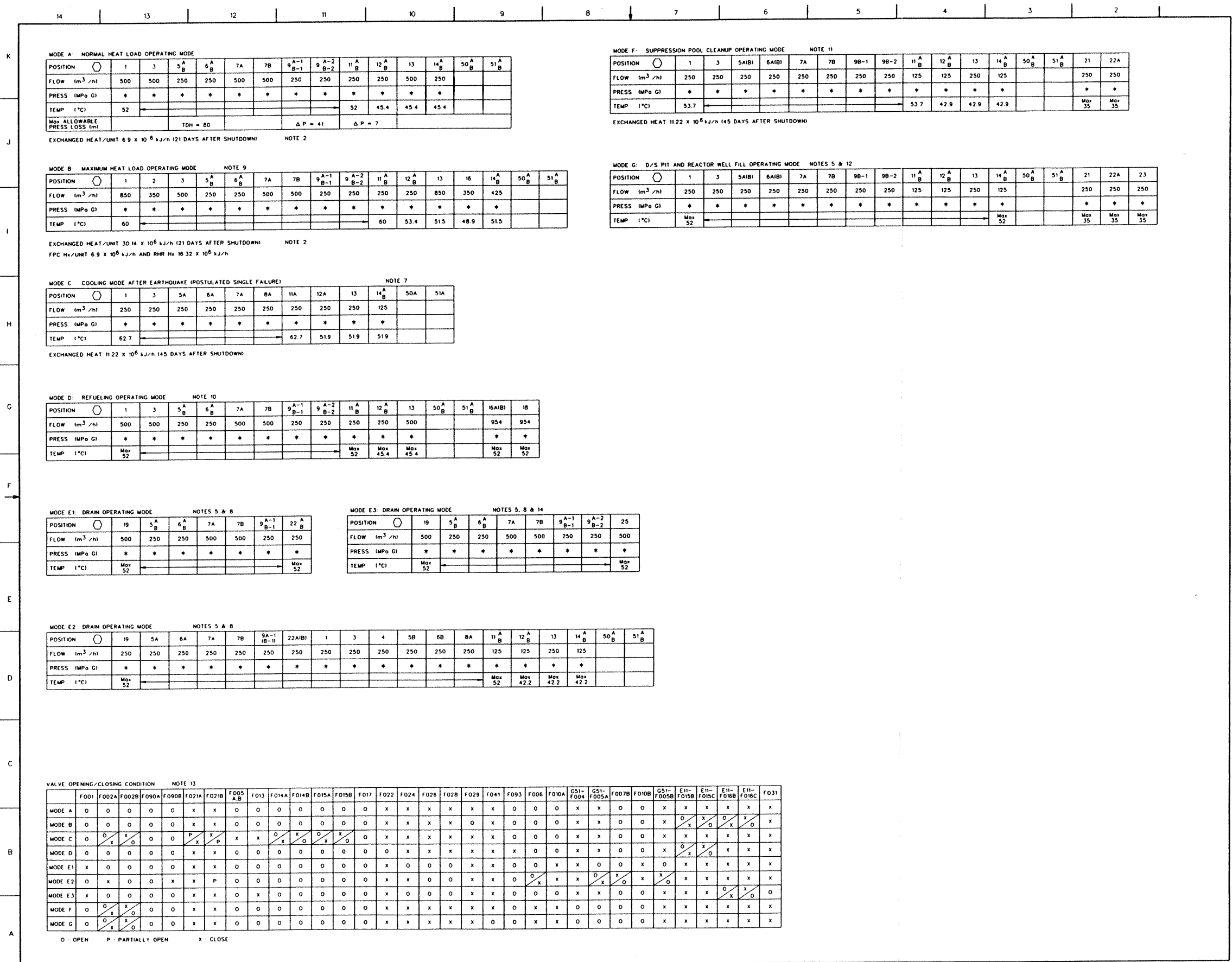
FIGURE 9.1-2 FUEL POOL COOLING AND CLEANUP SYSTEM PFD (Sheet 2 of 2) ABWR DCD/Tier 2 Rev. 0
