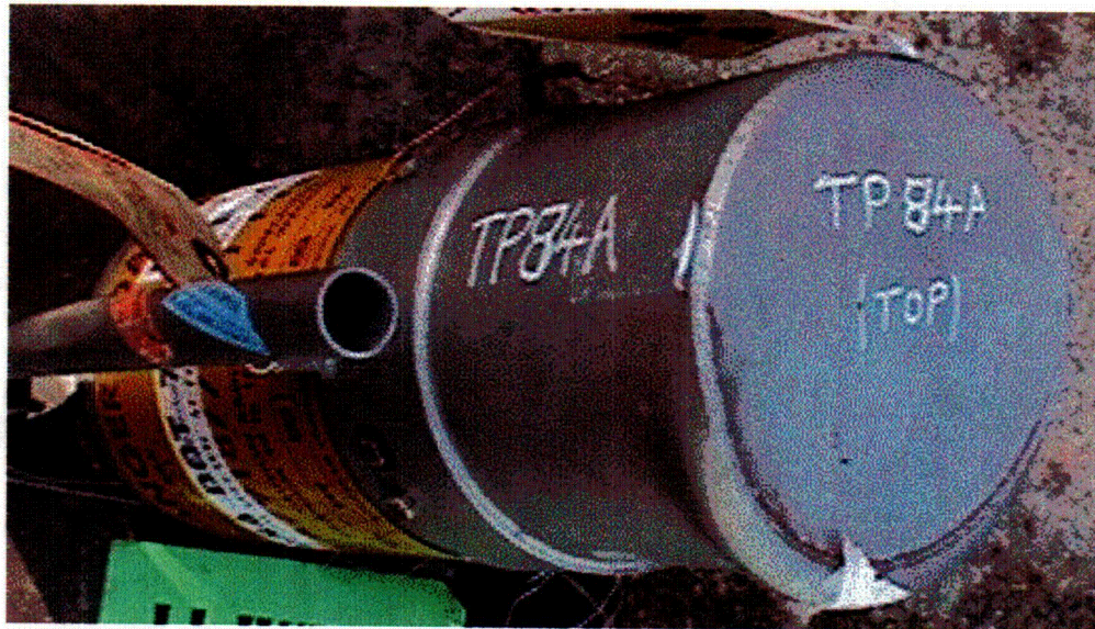
Figure 9: Buckling of top cover of TP84(A) after first 30 foot drop attempt
