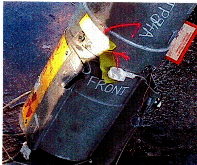
Figure 14: Puncture test damage to TP84(A)
