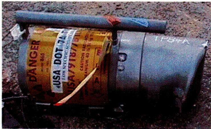
Figure 11: Damage to TP84(A) following second 30 foot drop attempt
