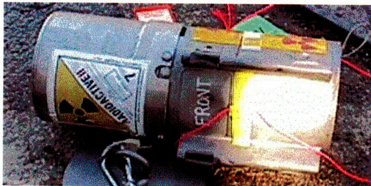
Figure 16: Puncture test damage to TP84(B) following drop 1
