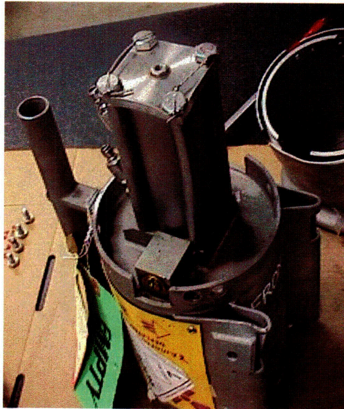
Figure 19: Damage to TP84(A) actuator assembly
