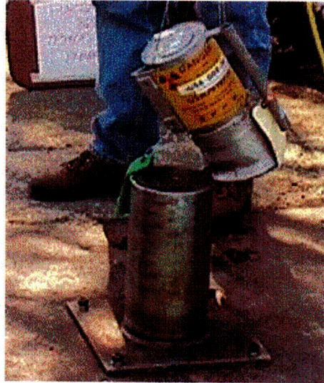
Figure 13: Puncture test set-up for TP84(A)
