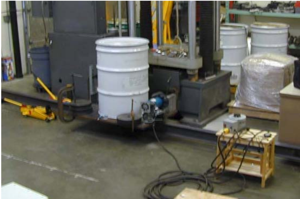
Figure 2.12.1-1 - Vibration Test Setup
