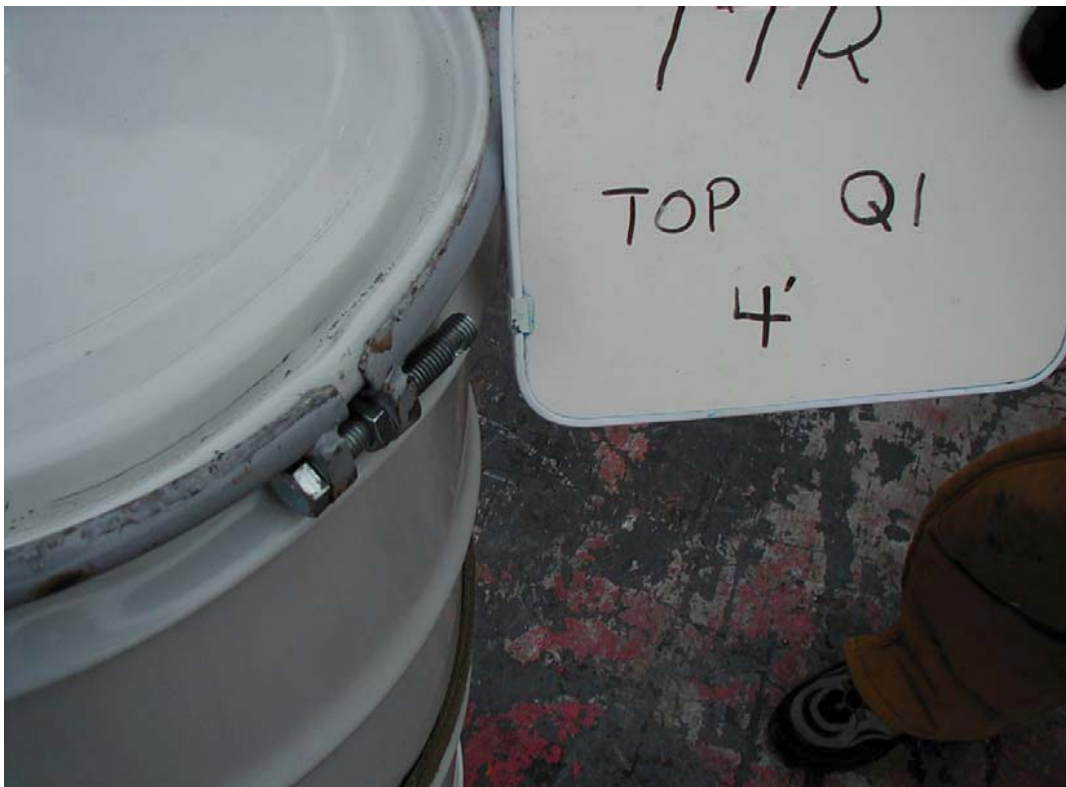
Figure 2.12.1-3 - Damage from CG over Corner Four-Foot Free Drop
