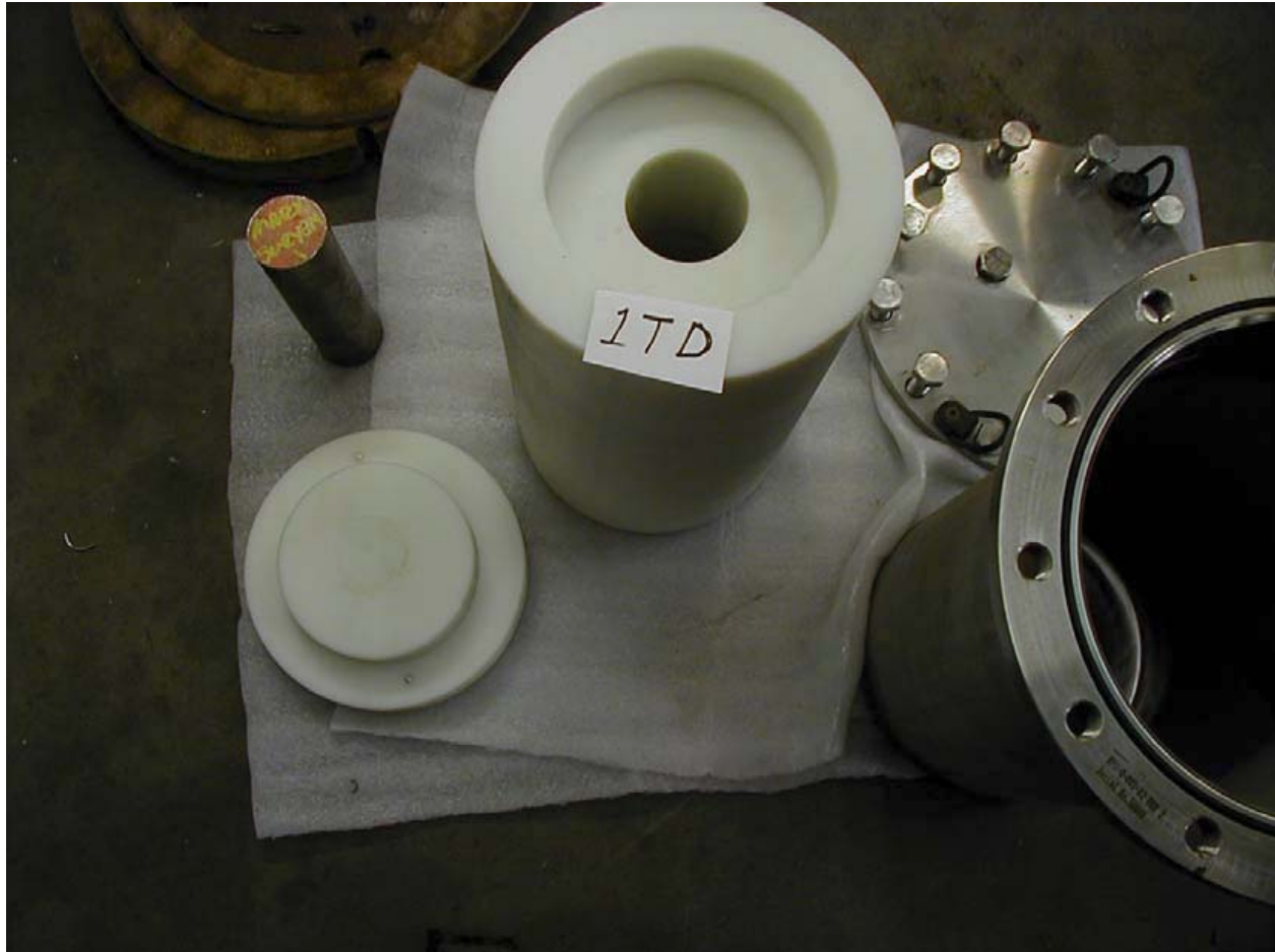
Figure 2.12.1-7 - Pipe Component Internals After All Drops
