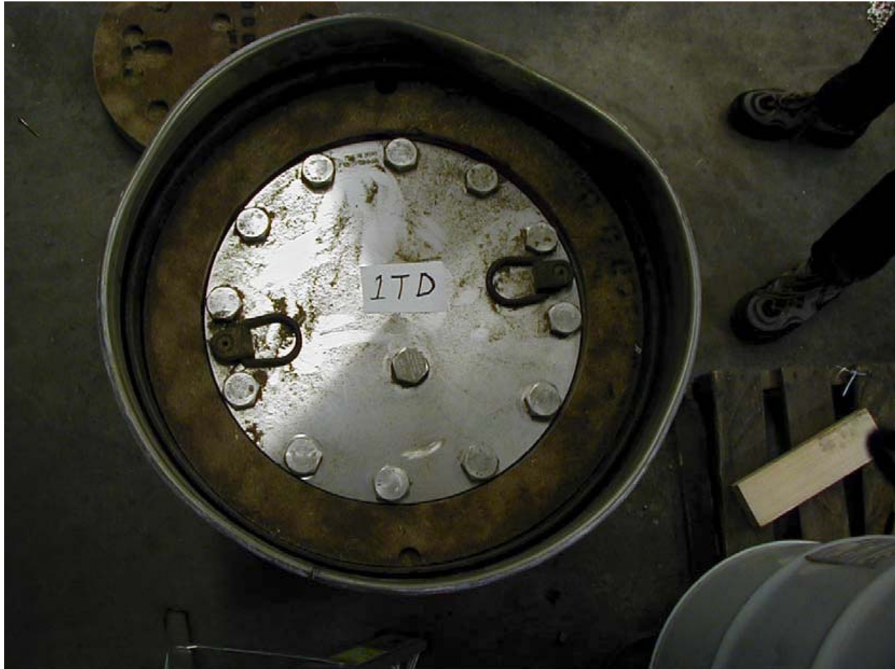
Figure 2.12.1-6 - Lid Removed After All Drops
