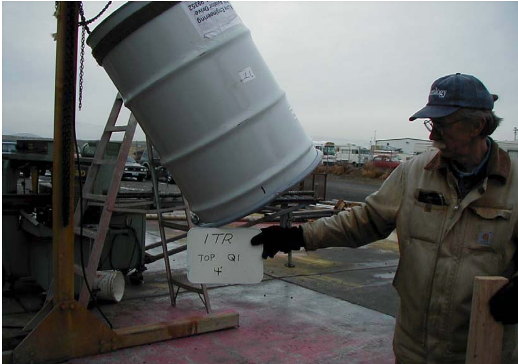
Figure 2.12.1-2 - S300 CG over Corner Four-Foot Free Drop
