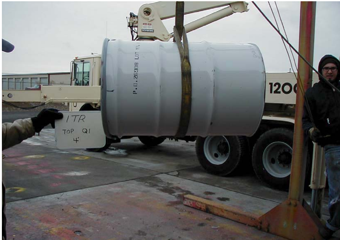
Figure 2.12.1-4 - S300 Side Four-Foot Free Drop
