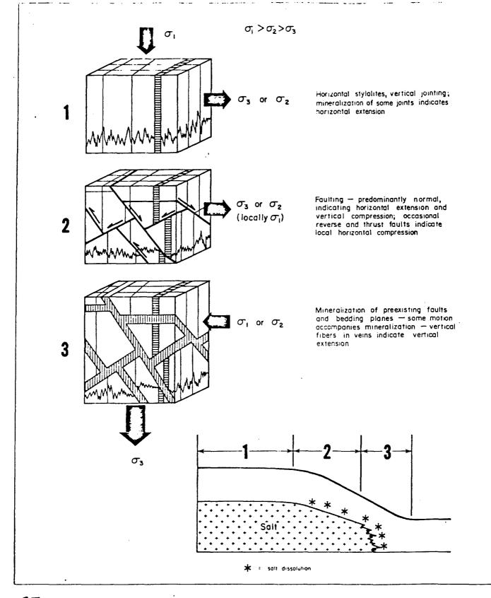
5/ide 27 . Conceptual model of brittle deformation above dissolution zones. Stage 1 represents normal burial; Stage 2 represents horizontal extension as a precursor to dissolution collapse; Stage 3 represents collapse (from Goldstein, 1982).
