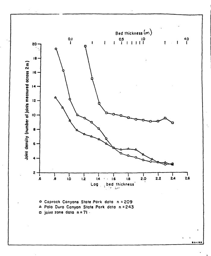
gure 8 Graph showing weighted joint density versus log of bed thickness for data from aprock Canyons State Park, Palo Duro Canyon State Park, and joint zones at both parks.
