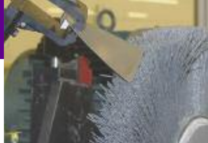
Deburring the tip of a turbine blade.
