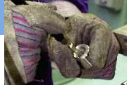
Deburring the I.D. of a small machined part.
