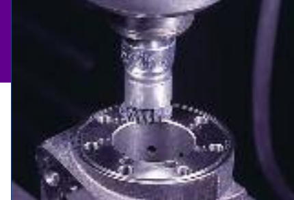
Blending tool marks on a hydraulic component.
