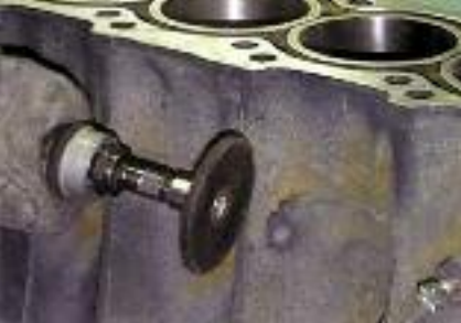
Removing flash from a sand-cast iron engine block.
