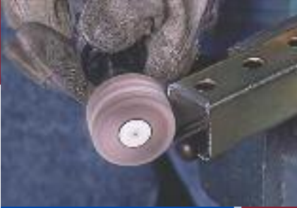
Deburring perforated steel channel after saw-cut.
