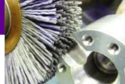
Deburring the edges of a machined aluminum component.
