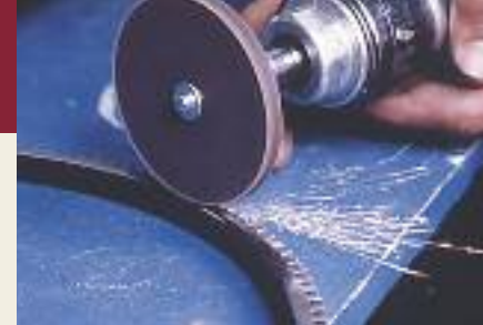
A unitized wheel deburring a ring gear.
