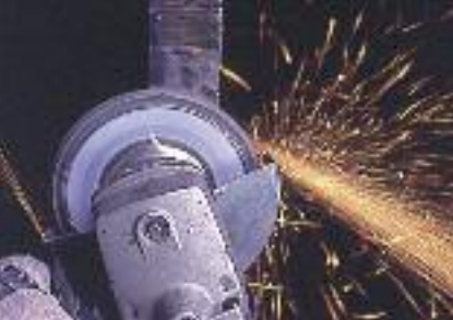
Blending and finishing edges of a flame-cut steel part.
