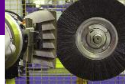
Deburring a vane section for a jet engine.
