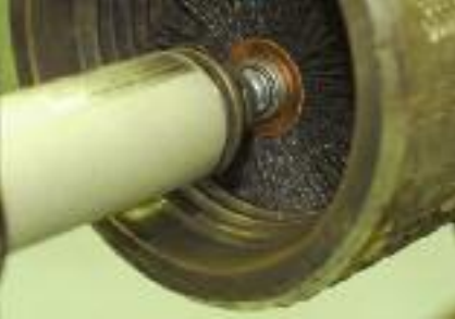
Cleaning internal threads inside a valve.
