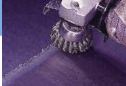
Removing slag from a flame-cut steel plate.
