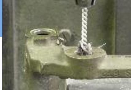
Removing zinc coating from holes in a brake bracket.
